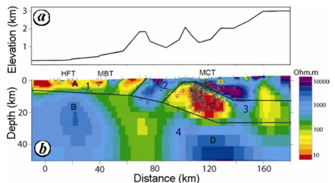
**Figure 1.** Topography (a) and 2D crustal electrical resistivity structure (b) along a profile in the Garhwal Himalaya (modified after Israil *et al.*<sup>23</sup>). Simplified crustal model (solid black lines) used in the present work is superimposed and four zones (1–4) have the resistivity of 25, 5000, 10 and 1000 Ohm.m respectively. HFT, Himalayan Frontal Thrust; MBT, Main Boundary Thrust, and MCT, Main Central Thrust. A, B, C, D indicate the major geoelectrical features of the model.
