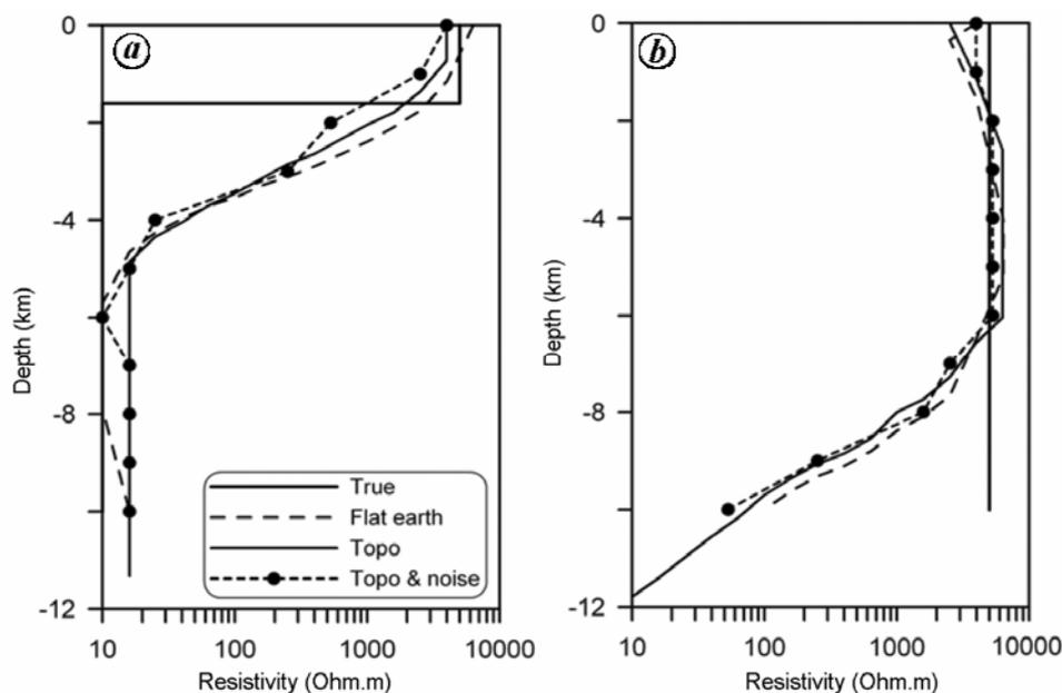
**Figure 4.** Variation of resistivity with depth at (a) site-12 and (b) site-15 after inversion of noise-free data assuming flat earth model (dashed curve) and topography model (solid curve). The results after inversion of noisy data with 10% Gaussian noise for topography model are shown by dashed curve with solid circles. Thick solid line represents the true model ('True'). Thin solid curve represents the inverted model including topography ('Topo').
