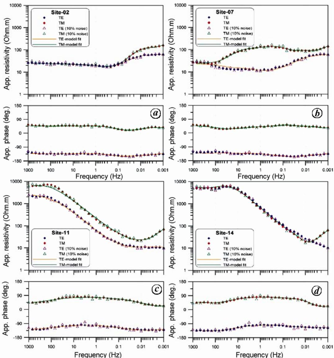
**Figure 2.** Synthetic apparent resistivity and phase response at four sites for the simplified crustal model with topography shown in Figure 1. Filled and open symbols represent noise-free and noisy (with 10% Gaussian distribution) data respectively. These data have been used as observed responses for the flat earth and topography models. Solid curves show the response of the best-fit model for the noisy data. Locations of the sites are marked in Figure 3.
