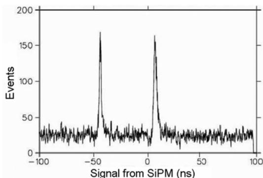
**Figure 3.** Histogram output from one of the SiPMs that was positioned to see maximum Cherenkov light for an angle setting of  $7.5^\circ$  of radiator with respect to the beam. The two peaks are due to triggering from both the leading edge and the trailing edge.
