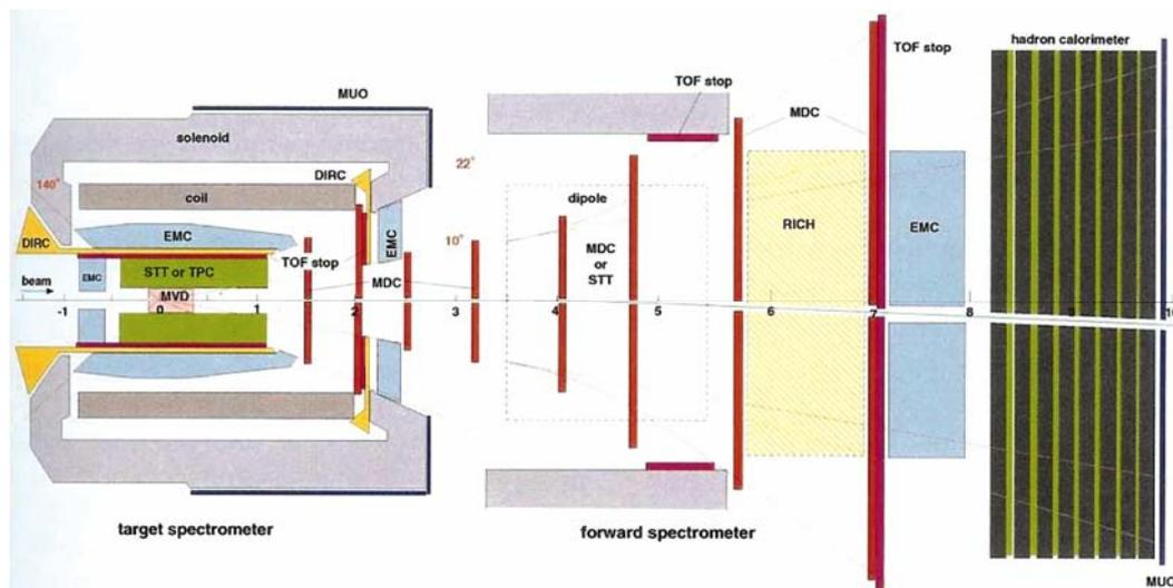
**Figure 1.** A schematic view of the PANDA detector. The HESR beam enters the detector from the left, interacts with the target at 0 m on the horizontal scale. The surrounding and forward detectors are indicated as MVD, Micro vertex detector; STT, Straw tube tracker; TPC, Time projection chamber; TOF, Time-of-flight stop counters; DIRC and RICH, Cherenkov counters; EMC, Electro magnetic calorimeter; MDC, Multi-wire drift chamber; MUO, Muon counter and hadron calorimeter<sup>1</sup>.
