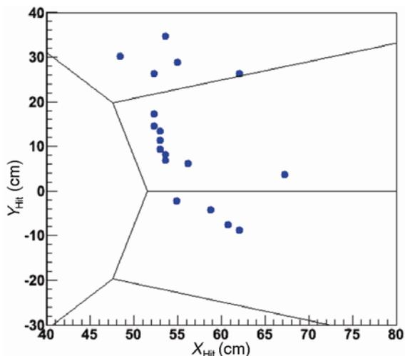
**Figure 4.** The expected ring structure in the photon detector plane for an incident kaon with momentum 2 GeV/c.
