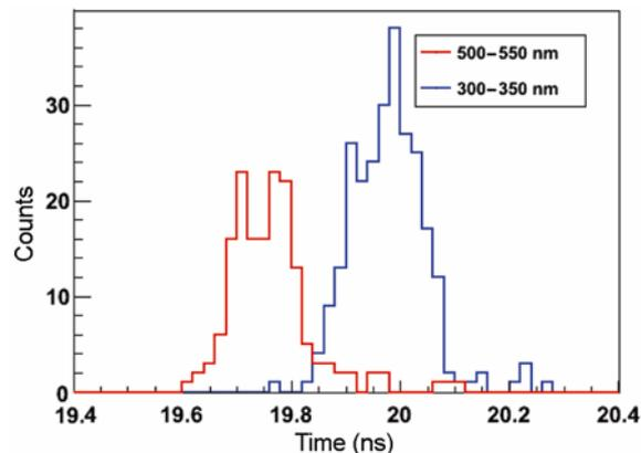
**Figure 5.** Time distribution for the different wavelength band for an incident kaon with momentum 2 GeV/c.
