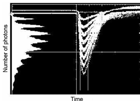
**Figure 2.** A typical SiPM spectrum from Hamamatsu MPPC triggered by laser light. Different peaks correspond to different photo peaks, hence, the number of pixels fired. In this case, up to eight photon peaks are seen. Photograph is taken from digital oscilloscope with the histogramming mode on.
