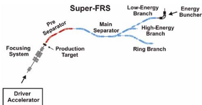
**Figure 2.** Schematic layout of the Super-FRS, the position of high-energy, low-energy and the ring branch that constitute the NuSTAR.
