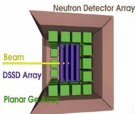
**Figure 5.** Experimental set-up of DESPEC showing the active target surrounded stack of planar HPGGe strip detectors and neutron detectors.
