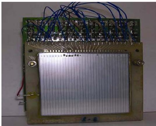
**Figure 8.** Si strip detectors developed by BEL–BARC collaboration and used for heavy fragment detection in fission experiments at TIFR–BARC pelletron facility.
