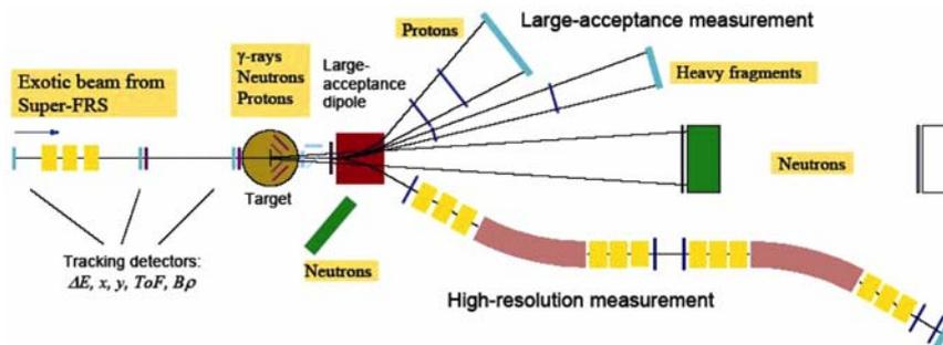
Figure 4. Schematic of the R<sup>3</sup>B set-up for high-acceptance and high-resolution measurements for the study of RIBs through reactions at relativistic energy.
