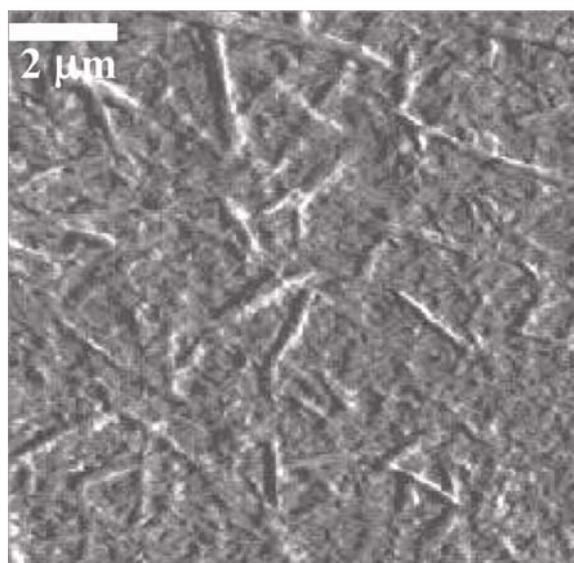
**Figure 1.** Atomic force microscopic images of cellulose whiskers obtained from acid hydrolysis of cellulose paper.
