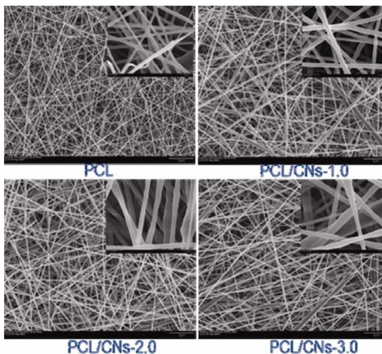
**Figure 4.** Field emission scanning electron microscopic (FESEM) images of PCL and PCL/CN electrospun fibres.
