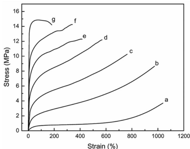
**Figure 2.** Stress–strain curves of water-borne polyurethane (WPU)/cellulose nanocrystal (CN) nanocomposite films having different CN contents: a, 0 wt%; b, 5 wt%; c, 10 wt%; d, 15 wt%; e, 20 wt%; f, 25 wt% and g, 30 wt%. Reprinted with permission from Kim *et al.*<sup>2</sup>. Copyright 2007 American Chemical Society.
