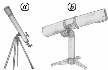
Figure 4. Simplest examples of (a) alt-azimuth and (b) equatorial mounts.
