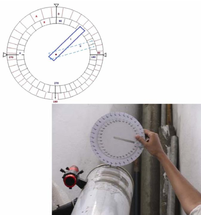
**Figure 6.** A device for helping amateur astronomers to assist in the alignment of (equatorial mount) telescopes. A modification connects this into a Dhruvabhrmaka Yantra according to the description.
