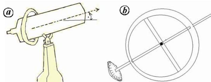
Figure 5. The equatorial mount (a) and comparison to Chakra Yantra (b).
