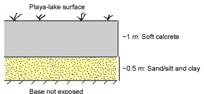
**Figure 4.** Representative stratigraphic section showing soft calcrete horizon at Lachhri.
