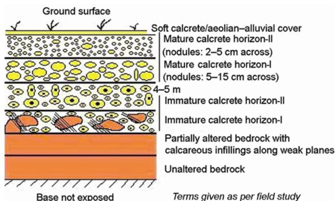
**Figure 3.** Generalized integrated stratigraphic section showing various types of calcrete horizons present in the region, depicting the different stages of calcrete development.
