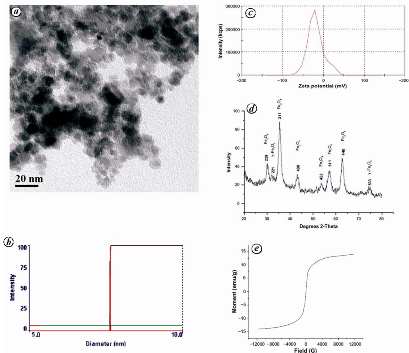
**Figure 1.** *a*, Transmission electron microscopic (TEM) image of  $\text{Fe}_3\text{O}_4$  nanocrystals taken at 120 kV in Joel TEM machine. *b*, Dynamic light scattering data of magnetic nanocrystals showing the degree of polydispersity. *c*, Zeta potential of magnetic nanoparticles ( $-19.08$  mV). *d*, X-ray diffraction pattern of iron nanoparticles. *e*, Magnetization of nanoparticles as measured by vibrating sample magnetometry at room temperature.
