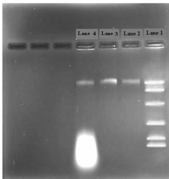
**Figure 2.** Agarose gel electrophoresis of bacterial genomic DNA extracted using bare magnetic nanoparticles (lane 2), by commercial DNA extraction kit (Chromous Biotech; lane 3) and phenol–chloroform method (lane 4). Lane 1, DNA molecular weight marker (lambda phage DNA/*Hind*III digest).
