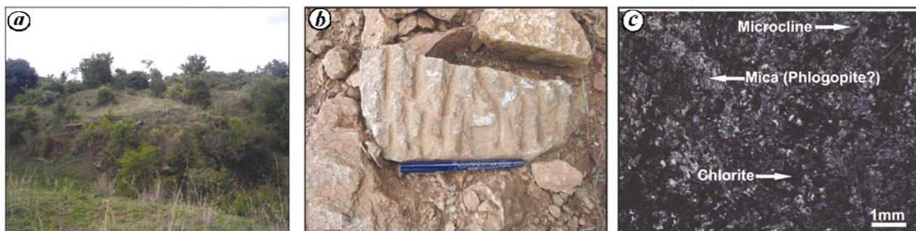
**Figure 2.** *a*, View of the Hoysala stone quarry at Pushpagiri (see Figure 1 for location). *b*, Rock specimen of chlorite schist from the quarry. Note the chisel marks of the Hoysala craftsmen. *c*, Microscopic view of the thin section (under cross-nicols) of a rock specimen from the quarry.
