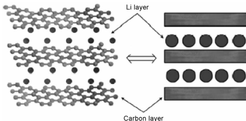
**Figure 1.** Schematic diagram showing the intercalation of graphite with lithium.
