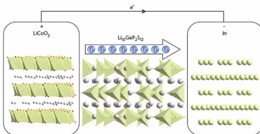
**Figure 2.** Schematic diagram of the all-solid-state lithium-ion battery reported by Kamaya *et al.*<sup>4</sup>. An all-solid-state battery with the structure  $\text{LiCoO}_2/\text{Li}_{10}\text{GeP}_2\text{S}_{12}/\text{In}$  (from Masquelier<sup>3</sup>, reprinted with permission from Nature Publishing Group).
