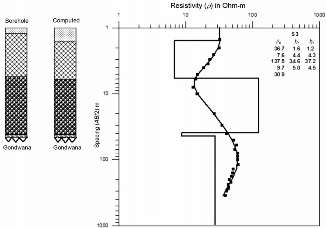
**Figure 3.** Comparison of computed thickness of layers ( $h_c$ ) with the thickness obtained from bore well ( $h_b$ ) at site S3, Kotwalbardi village.
