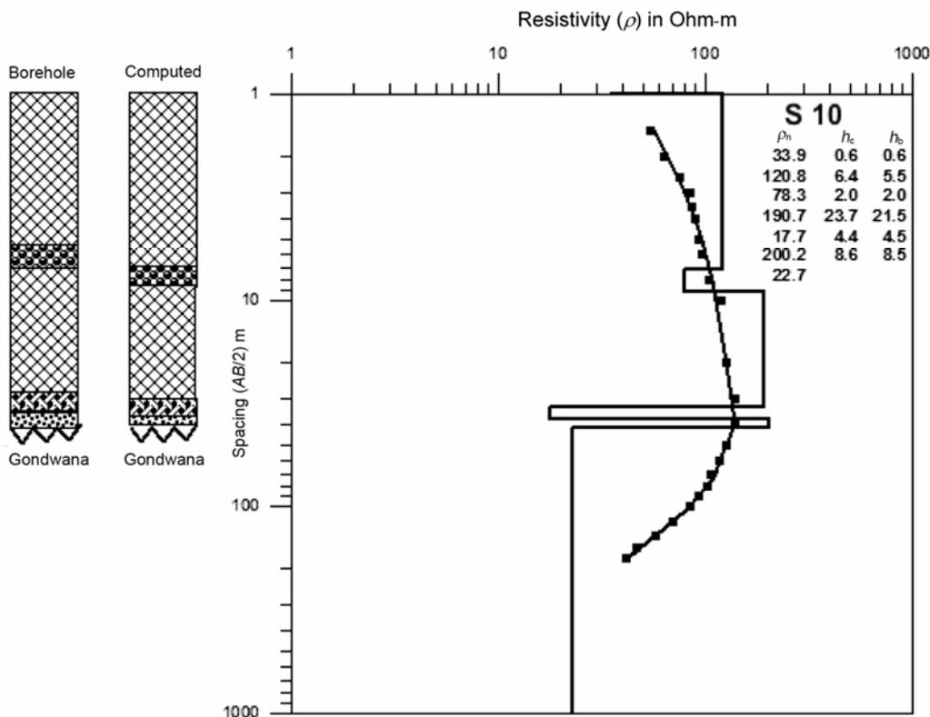
Figure 5. Comparison of computed thickness of layers ( $h_c$ ) with the thickness obtained from bore well ( $h_b$ ) at site S10, Raulgaon village.
