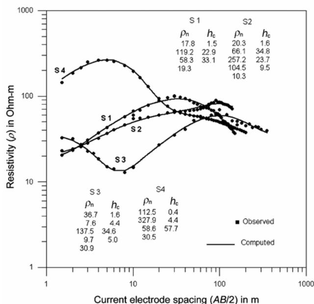
Figure 2. Resistivity models for sites S1–S4, Kotwalbardi village.
