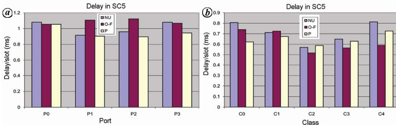
Figure 5. Delay rate for various traffic patterns for service class 5 using first-fit wavelength assignment algorithm (a) and reservation bit algorithm (b).
