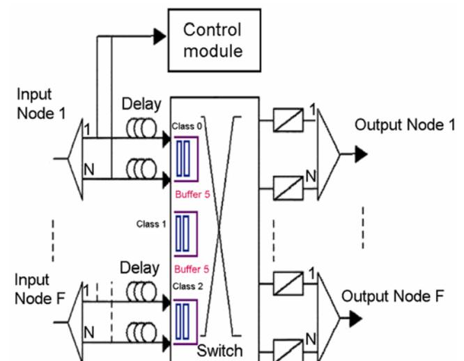
**Figure 1.** Architecture of the optical packet switching network with buffers.
