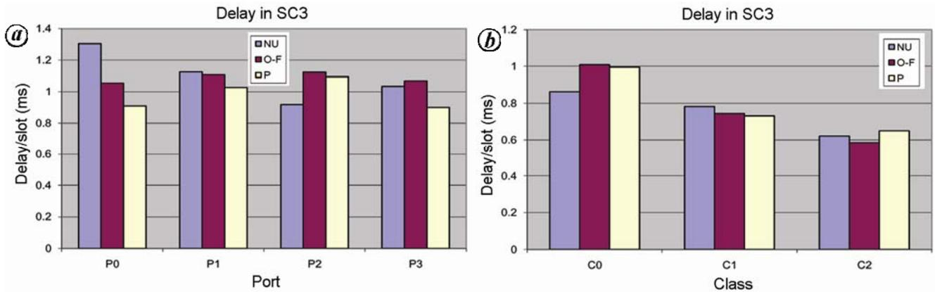
**Figure 3.** Delay rate for various traffic patterns for service class 3 using first-fit wavelength assignment algorithm (a) and reservation bit algorithm (b).
