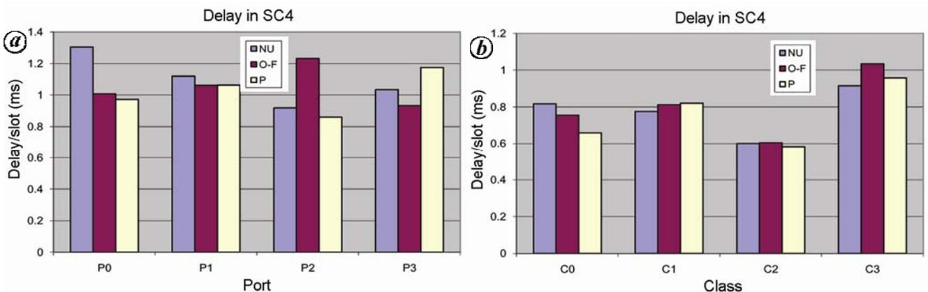
**Figure 4.** Delay rate for various traffic patterns for service class 4 using first-fit wavelength assignment algorithm (a) and reservation bit algorithm (b).
