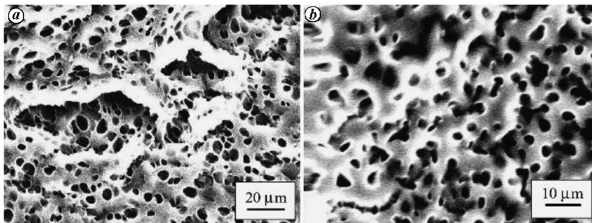
**Figure 2.** Schematic view of (a) SEM images of PDLC without nanoparticles (NPs) ( $\phi_p = 40$  vol%), (b) PDLC doped with  $\text{Sb}_2\text{O}_5$  NPs ( $\phi_p = 38$  vol%,  $\text{Sb}_2\text{O}_5 = 3$  vol%). (Reproduced from Yaroshchuk *et al.*<sup>15</sup> with permission from Elsevier Science Ltd, The Netherlands.)
