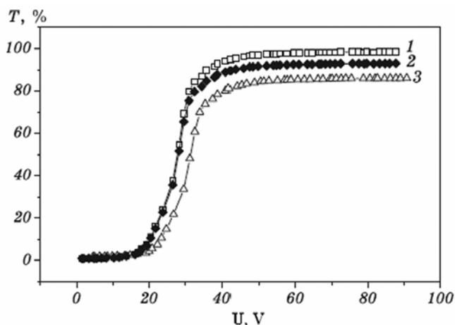
**Figure 3.** View of the  $T$ - $UV$  curves for the non-doped and NP-doped PDLC composites. (1)  $\phi_p = 40$  vol%;  $\phi_{NP} = 0$  vol%; (2)  $\phi_p = 39$  vol%;  $\phi_{NP} = 1$  vol% ( $\text{SiO}_2$  NPs) and (3)  $\phi_p = 39$  vol%;  $\phi_{NP} = 1$  vol% ( $\text{Sb}_2\text{O}_5$  NPs). (Reproduced from Yaroshchuk *et al.*<sup>15</sup> with permission from Elsevier Science Ltd, The Netherlands.)
