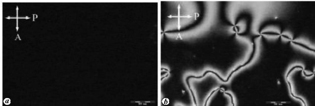
**Figure 4.** Polarizing optical microscopic views of the (a) 20 wt% polyhedral oligomeric silsesquioxane filled liquid crystal (LC) test cell and (b) LC test cell. Such cells were fabricated by two nontreated ITO-glass substrates and sandwiched between crossed polarizers. (Adopted from Kuo *et al.*<sup>25</sup> with permission from American Institute of Physics, USA.)
