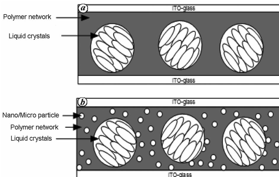
**Figure 1.** Schematic view of (a) conventional polymer-dispersed liquid crystal (PDLC) film, and (b) nanoparticle-doped PDLC film.
