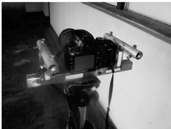
**Figure 1.** The Canon Rebel *XTi* digital camera mounted on a horizontal metal frame, flanked by tubes housing the laser pointers 20 cm apart.
