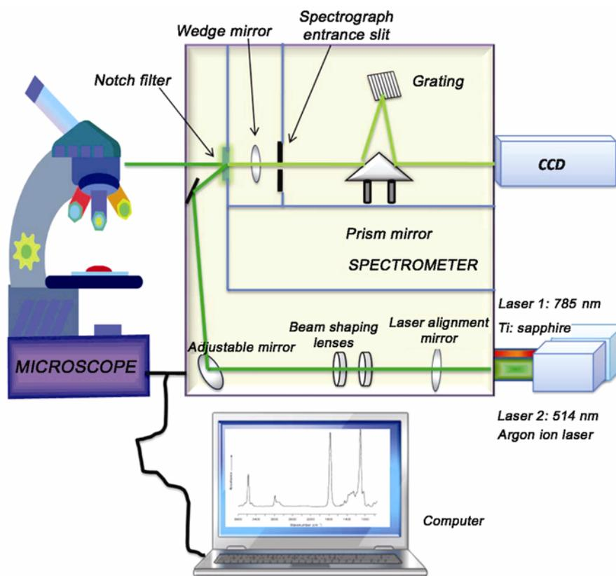
Figure 3. Ray diagram of Raman microspectrometer.
