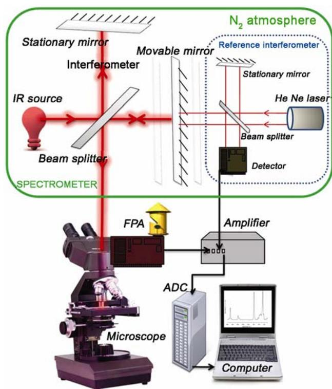
**Figure 4.** Ray diagram of FTIR microspectrometer.
