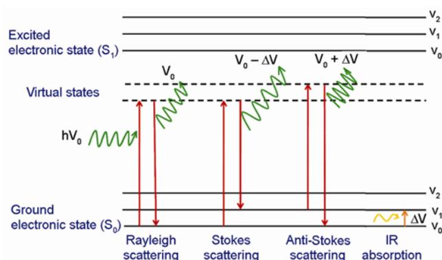
**Figure 2.** Energy-level diagram representing Raman and infrared processes.
