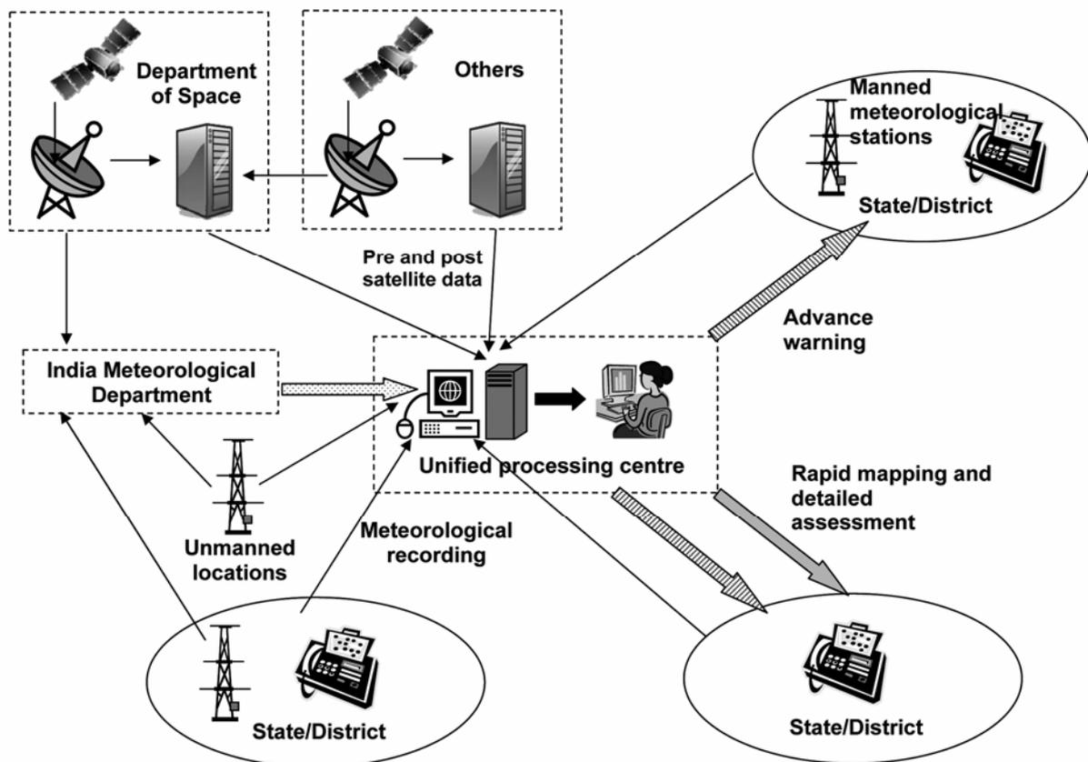
Figure 6. A framework for the Unified Processing Centre for advance warning system and post-disaster assessment.
