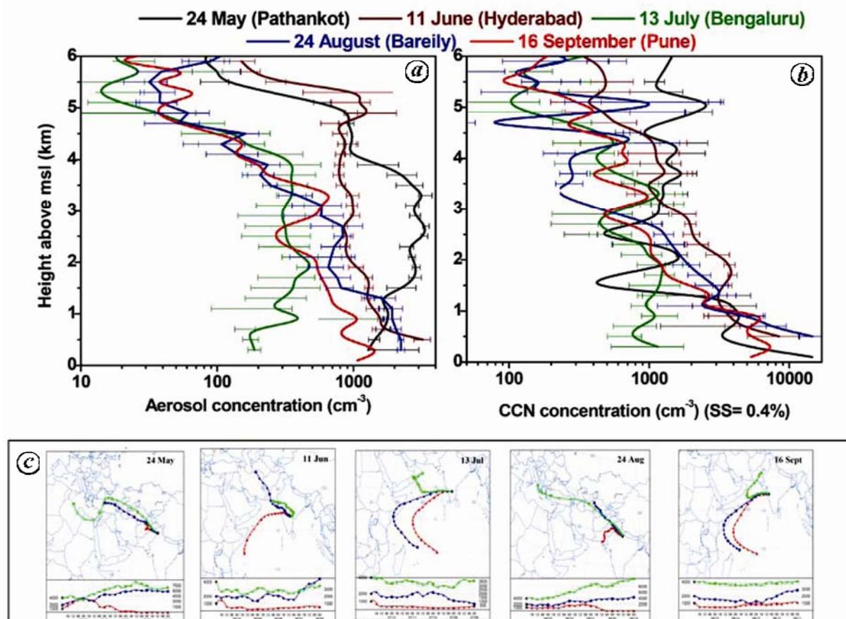
**Figure 4.** Vertical distribution of aerosol concentrations from (a) aerosol and (b) CCN concentration at different locations. Each point corresponds to aerosol measurements averaged for every 200 m level and the error bar corresponds to variation within 200 m. All data are cloud-screened. (c), The Hysplit backward (5 days) trajectories for the five cases at the respective IOP locations.
