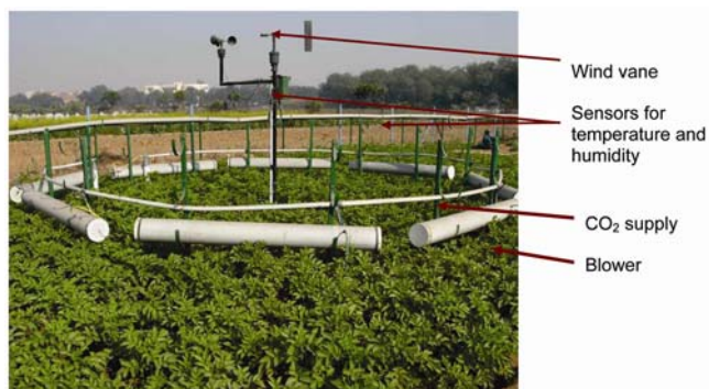
Figure 1. Free-air CO 2 enrichment system in Indian Agricultural Research Institute, New Delhi.
