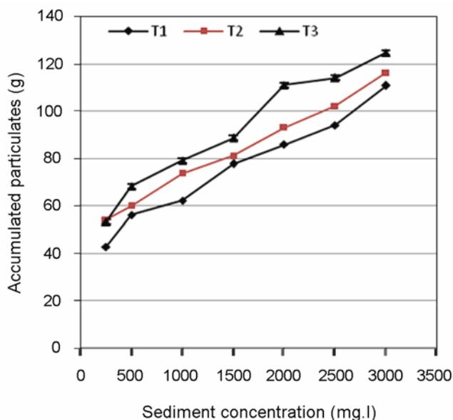
Figure 5. Suspended particulates retained by top layer (10 cm) of different CS beds.
