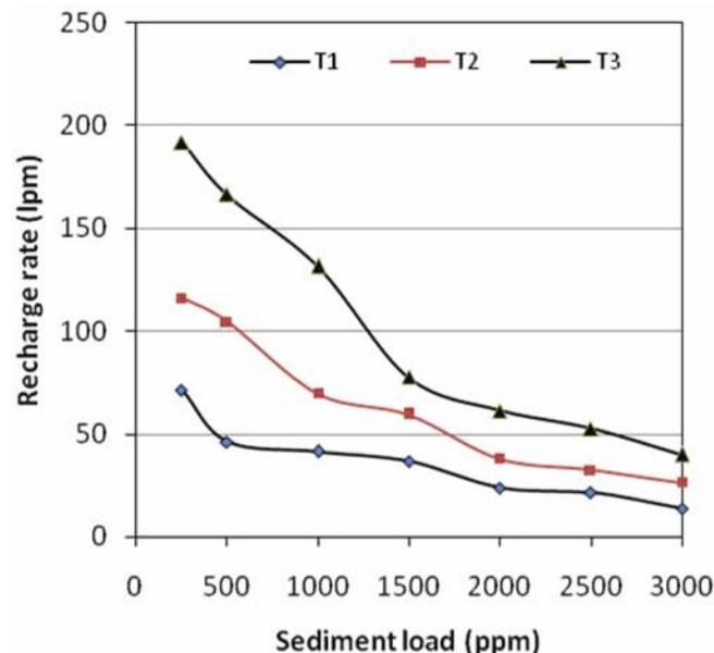
Figure 6. Effect of inflow water sediment load on average recharge rate of different coarse media.
