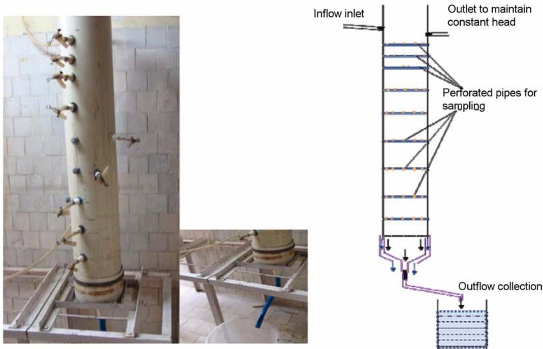
**Figure 1.** Photograph and diagram of experimental column used in the laboratory study.
