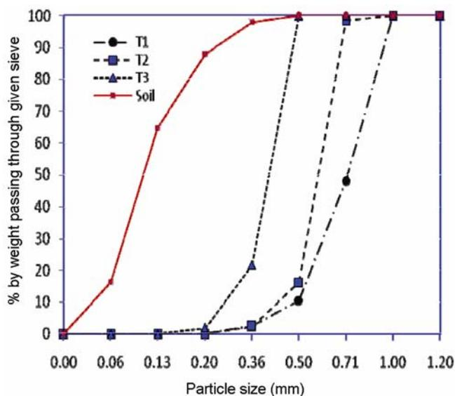
**Figure 2.** Gradation curve for the materials used in the laboratory study.
