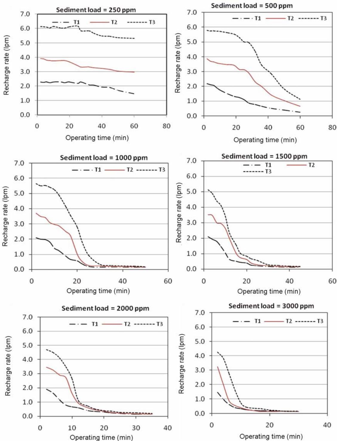
Figure 7. Effect of operating time on performance of different CS beds.
