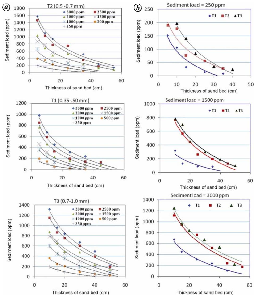
**Figure 4.** a, Effect of thickness of filtering medium and sediment concentration of influent water on sediment load of filtered water under different coarse sand beds. b, Effect of thickness of filtering medium and CS beds on sediment load of filtered water under varying inflow water sediment loads.
