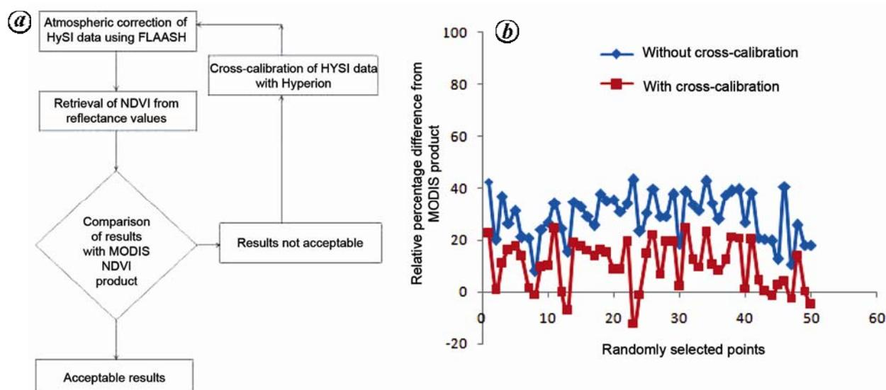
**Figure 2.** *a*, Atmospheric correction of HYSI data using FLAASH. *b*, Relative percentage difference of NDVI from those of MODIS product before and after cross-calibration of HySI data.
