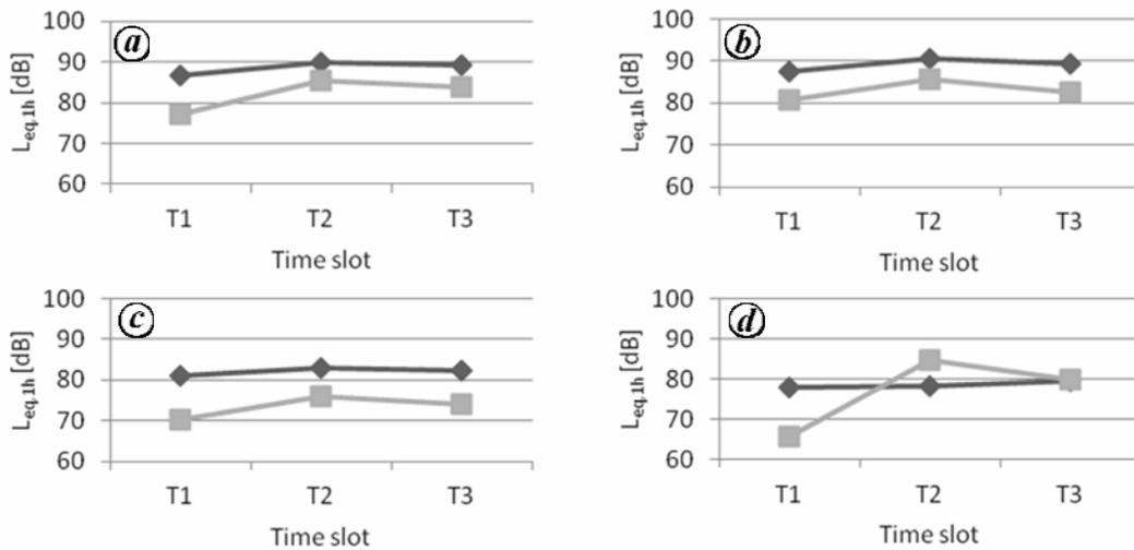
**Figure 5.** Four-days average  $L_{eq,1h}$  ( $L$ ) variation (in dB) for different time slots at locations: (a) A; (b) B; (c) C and (d) D. ♦ 63 Hz (black line); ■ 1 kHz (grey line).
