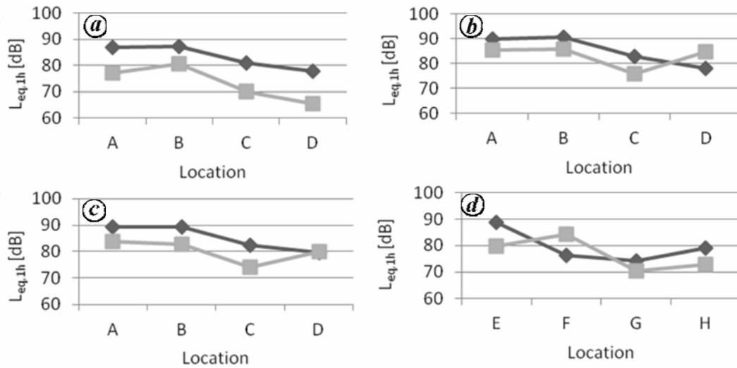
**Figure 4.** Variation of average  $L_{eq,1h}$  ( $L$ ) at different locations at sampling time slots: (a) T1; (b) T2; (c) T3 and (d) T4. ♦ 63 Hz (black line); ■ 1 kHz (grey line).
