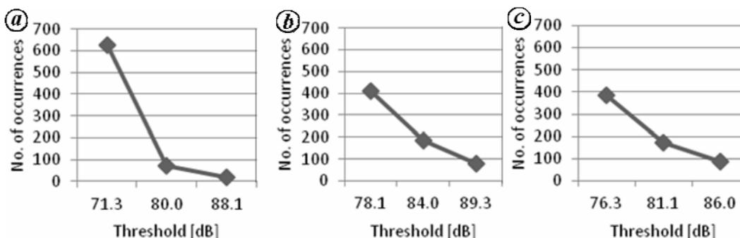
**Figure 8.** Average occurrences above thresholds for location A at time slots: (a) T1; (b) T2 and (c) T3 at 1 kHz.
