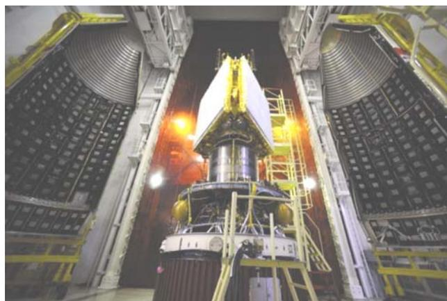
**Figure 4.** RISAT-1 before closure of heat shield.
