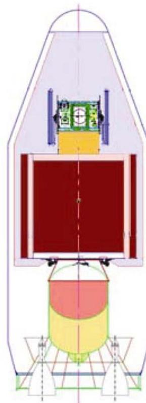
**Figure 3.** Accommodation of RISAT-1 within PSLV heat shield.
