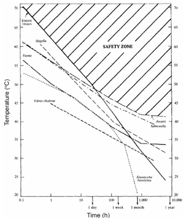
**Figure 1.** Temperature–time relationship for safe water pasteurization. The hatched area is the safe zone for all common pathogens. (Source: Feachem *et al.*<sup>10</sup>.)
