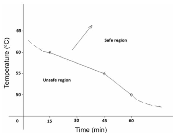
**Figure 2.** Temperature–time relationship for safe water pasteurization. In the area above the line no colony forming units of coliforms survive.
