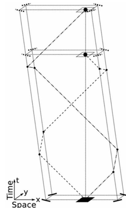
**Figure 4.** Minkowski space-time diagram of the experiment from the frame of reference of the observer (detector)<sup>5</sup>. The mirrors appear to move in the opposite direction from this frame. The inclination of the world lines followed by light to the horizontal plane does not change due to the constant speed of light. The world lines followed by the mirrors are at a greater angle due to their lower speed (i.e. they fall within the light cone).
