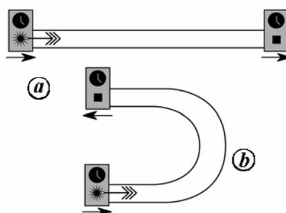
**Figure 1.** *a*, Simple set-up for measuring the speed of light in an inertial frame. *b*, Modified set-up<sup>4</sup>.
