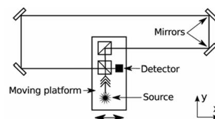
**Figure 3.** Schematic diagram of the experimental set-up used by Unnikrishnan<sup>3</sup>.
