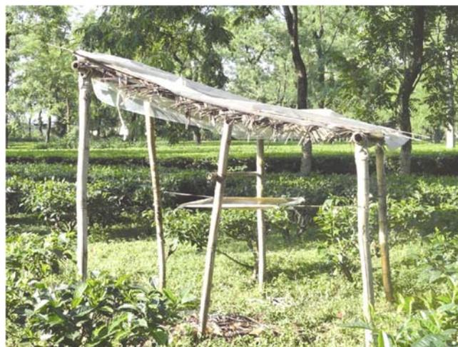
**Figure 1.** The light trap used in the present study.
