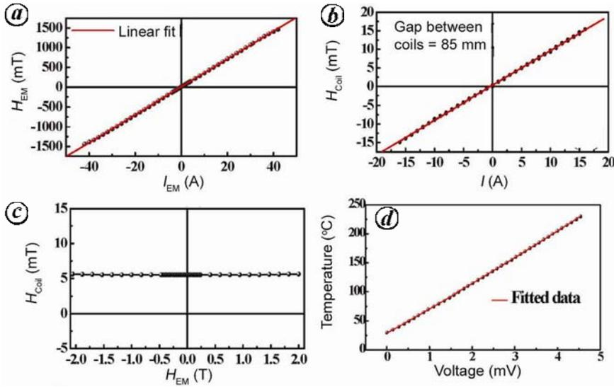
**Figure 6.** Calibration curve for (a) electromagnet field, (b) field produced by the Helmholtz coils, (c) effect of the electromagnet field on the Helmholtz coil field and (d) thermometer.
