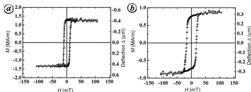
**Figure 10.**  $M$ – $H$  curve of  $(120 \pm 5)$  nm polycrystalline films of (a) Fe and (b) Co measured at  $30^\circ\text{C}$  (room temperature).
