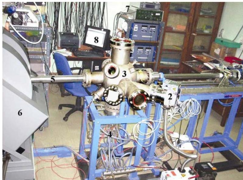
**Figure 4.** Image of the assembled CBM consisting of the manipulator with necessary electrical and water feed-through (1), high vacuum pumps (2), HV chamber (3), evaporator (4), non-magnetic hollow tube (5), electromagnetic system (6), CBM control unit (7) and personal computer for acquisition and processing data (8).
