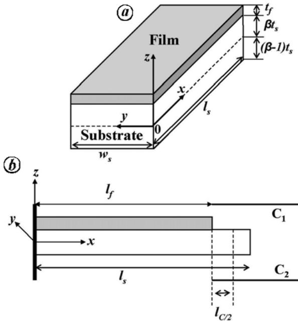
**Figure 7.** Film/substrate bimorph system with parameter notations and geometric directions of the cantilever substrate with thin film, where (a) shows the position of neutral plane and (b) shows the position of the cantilever substrate in capacitor plates.
