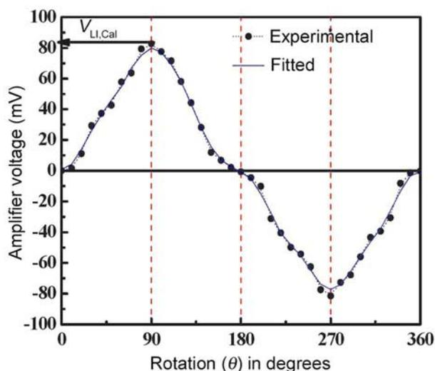
**Figure 5.** Calibration curve obtained by rotating the manipulator in steps through 360° to determine  $V_{Li,Cal}$ .
