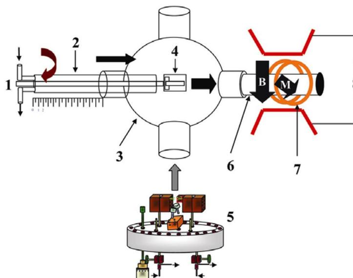
**Figure 2.** Schematic representation of the CBM set-up with (1) water and electrical feed-through; (2) manipulator rod; (3) high vacuum (HV) chamber; (4) CBM device; (5) evaporator; (6) non-magnetic hollow tube; (7) electromagnet pole pieces, and (8) pair of Helmholtz coils.
