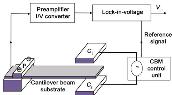
**Figure 1.** Schematic diagram of a cantilever beam magnetometer (CBM) device with electrical connections for the measurement of cantilever deflection.  $C_1$  and  $C_2$  represent the upper and lower capacitor plates and  $P$  is the substrate holder from where the signal is being derived.  $V_{LI}$  is the output lock-in-voltage.
