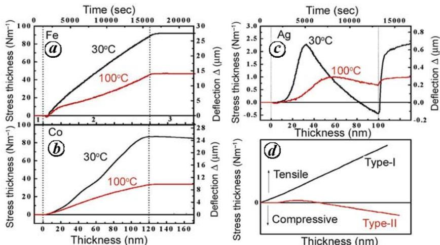
**Figure 8.** Experimental data of intrinsic stress in terms of stress–thickness product versus thickness (deposition time) for (a) Fe, (b) Co and (c) Ag measured at  $T_s = 30^\circ\text{C}$  (room temperature) and  $100^\circ\text{C}$ ; the dotted lines separate three regions according to the OFF (region 1 and 3) and ON (region 2) state of the shutter. (d) Schematic representation of the stress versus thickness curves of high melting point (type I) and low melting point (type II) materials.
