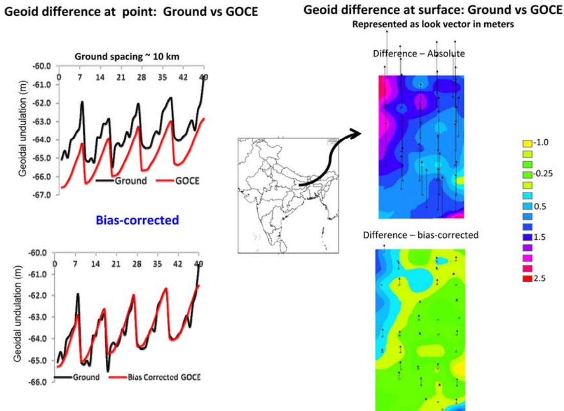
Figure 2. Difference between GOCE and ground data – absolute versus post bias correction of Kosi river basin, Bihar.
