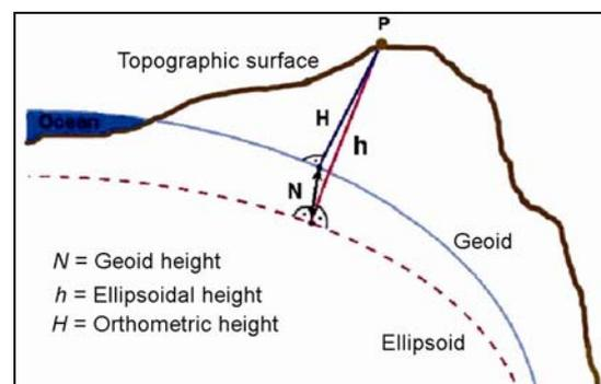
Figure 1. Relation between geoidal, ellipsoidal and orthometric heights.
