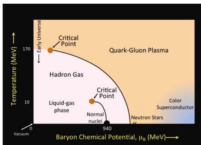
Figure 2. Schematic phase diagram of nuclear matter.
