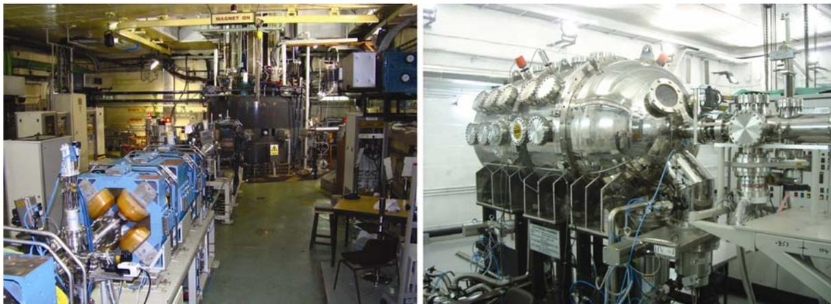
**Figure 3.** (Left) Photograph of the K-500 superconducting cyclotron along with the zero-degree beam line at the Variable Energy Cyclotron Centre, Kolkata. (Right) Photograph of a general-purpose scattering chamber in the beam line, which is designed to house complex detector arrays in vacuum.
