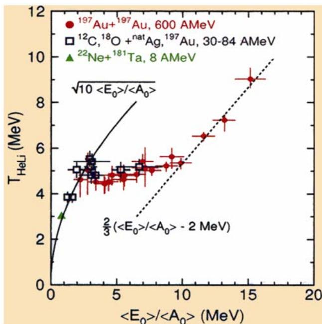
**Figure 4.** Caloric curve of nuclei determined by dependence of the isotope temperature on the excitation energy per nucleon<sup>14</sup>.
