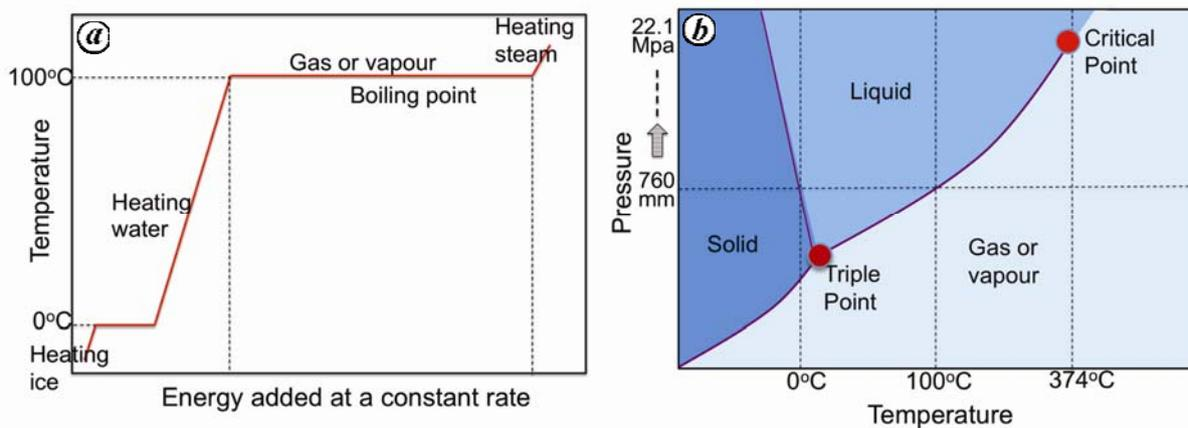
**Figure 1.** *a*, Phase change with additional energy to the system at atmospheric pressure. *b*, Phase diagram of water, showing the phases at various temperatures and pressures.
