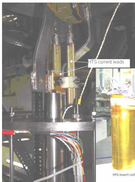
**Figure 1.** High Temperature Superconductor (HTS) insert coil and the full assembly ready for the test at 4.2 K.
