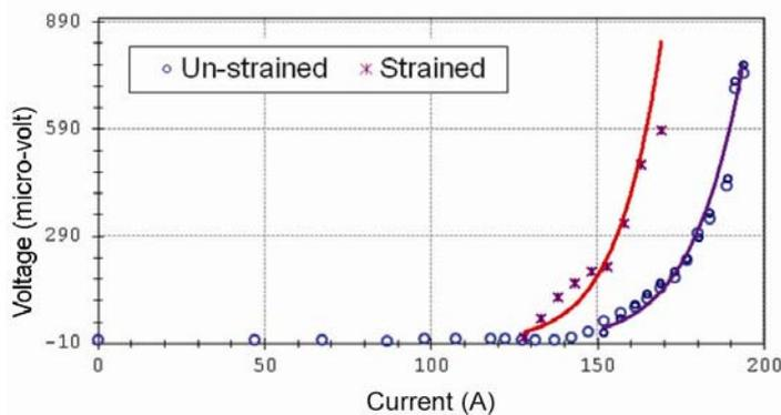
Figure 2. Degradation of critical current measured at 77 K due to tensile loading.
