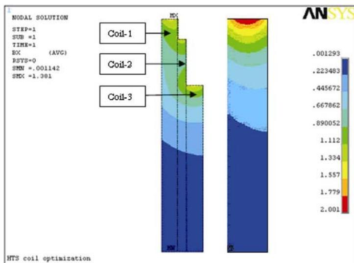
**Figure 3.** Reduction of radial component of magnetic field at the coil ends using three coils of different axial heights.
