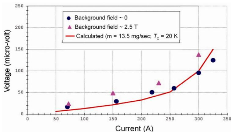
**Figure 5.** Voltage across resistive part of current lead during current ramping.
