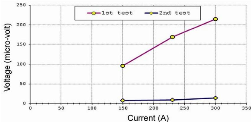
**Figure 6.** Voltage across the HTS part of current lead showing resistive during the first test.
