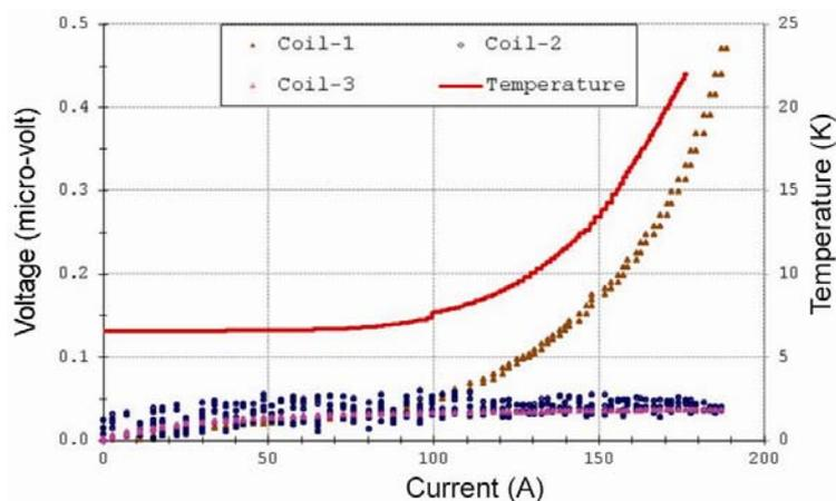
**Figure 4.** Voltage across the three coils during current ramping along with temperature rise.
