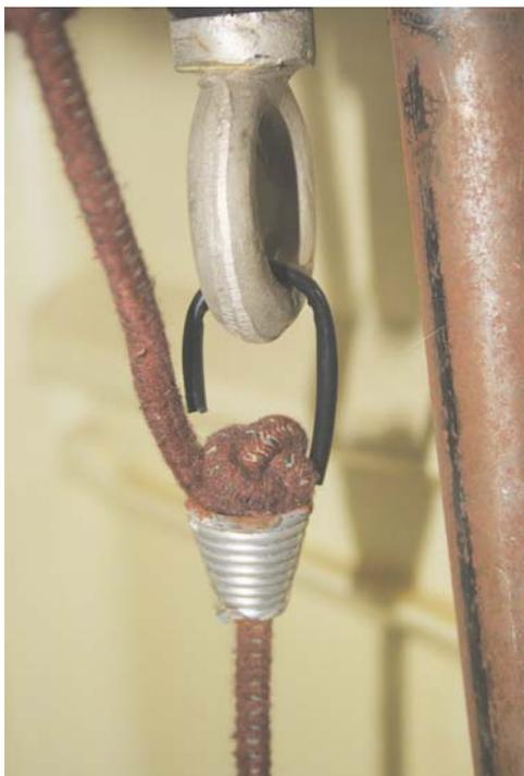
**Figure 3.** Use of a bungee chord for enhanced vibration isolation (photo: Pankaj Sekhsaria).
