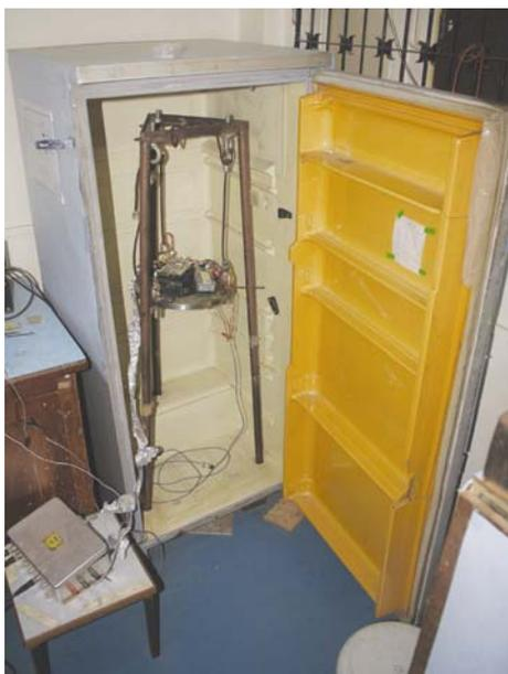
**Figure 1.** Scanning tunneling microscope installed inside the shell of a refrigerator after the compressor was removed (photo: Pankaj Sekhsaria).
