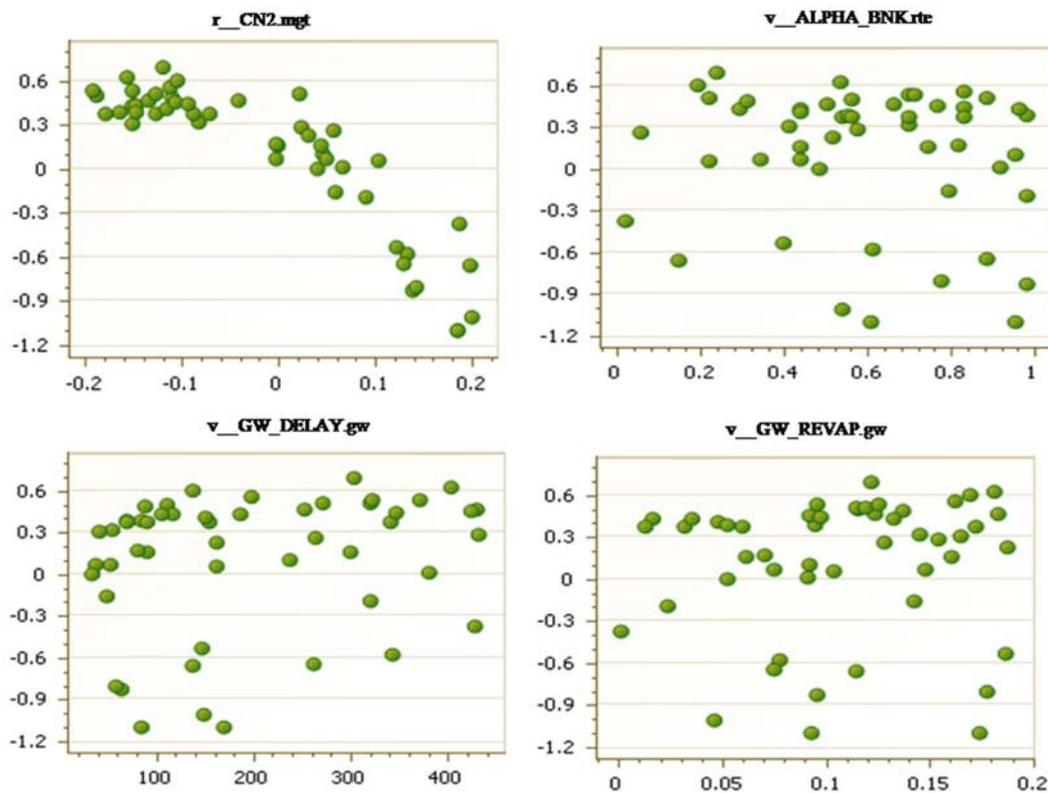
**Figure 6.** Plots showing most identified sensitive parameters during monthly calibration in GLUE.
