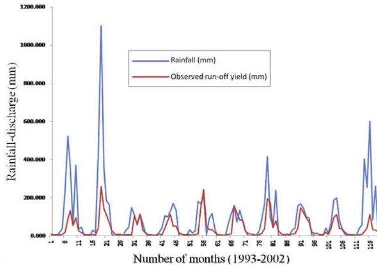
**Figure 7.** Monthly average comparison of rainfall and run-off at the outlet of the catchment during 1993–2002.
