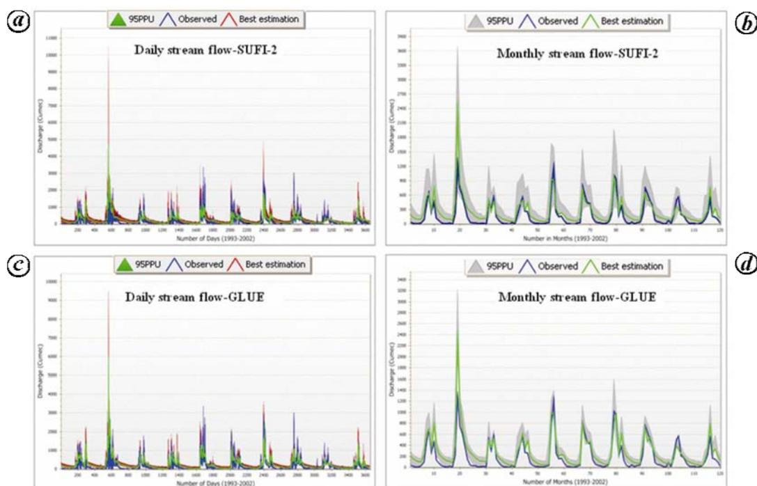
**Figure 9.** Daily (a, c) and monthly (b, d) stream flow calibration during 1993–2002.
