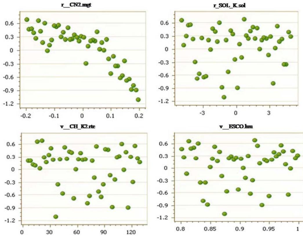
Figure 4. Plots showing most identified sensitive parameters during monthly calibration in SUFI-2.
