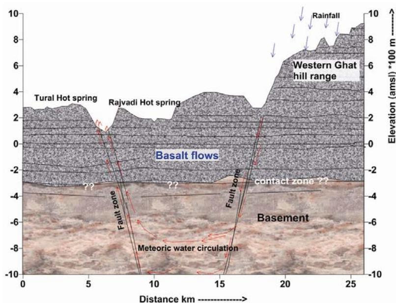
**Figure 4.** Hypothesized geological cross-section (west–east) associated with real topographic section indicating the possible mechanism of origin of hot springs with different circulation paths.
