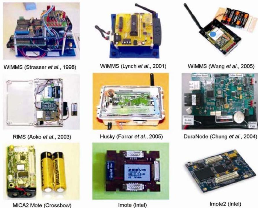
Figure 1. Various available wireless sensor platforms.
