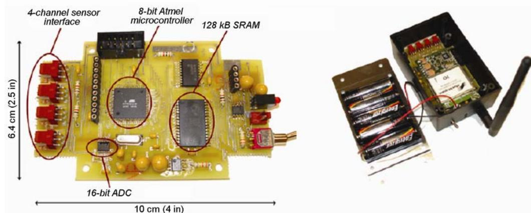
Figure 4. Wireless sensor prototype for structural health monitoring.
