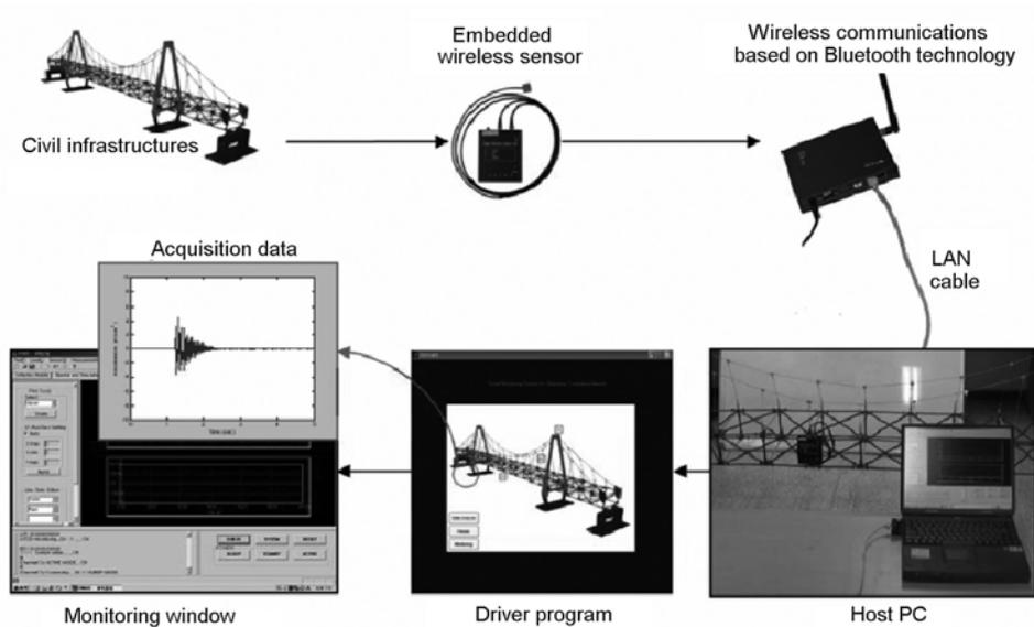
Figure 2. Ubiquitous smart monitoring test set-up.
