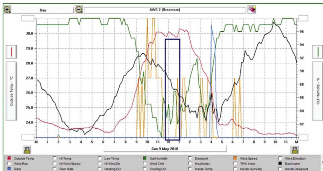
**Figure 2.** Screen shot of automatic weather station (AWS) data recorded on 9 May 2010 showing updraft events with simultaneous increase in relative humidity.
