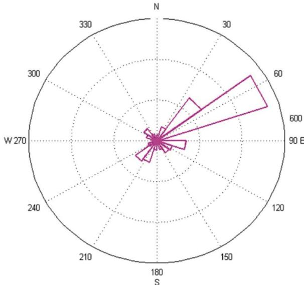
**Figure 3.** Wind rose diagram indicating wind direction from the coast during morning hours.
