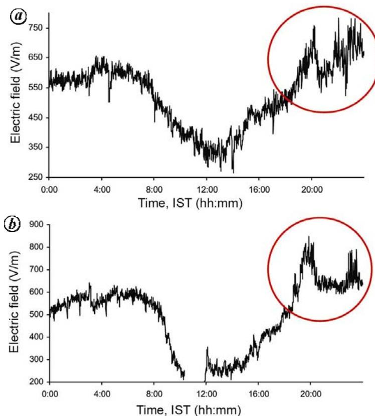
**Figure 11.** Electric field measured at Braemore on 7 May 2010 (a) and 5 May 2010 (b). Shown inside the circles are the transients associated with thunderstorm activity over the location.
