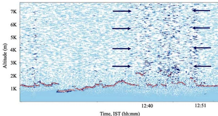
**Figure 7.** Ceilometer display showing particle distribution between 12:40 and 12:51 h. The vertical band-like structure between the arrows indicates the presence of water droplets.
