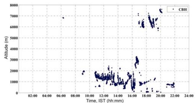
**Figure 6.** Ceilometer data recorded at Braemore on 9 May 2010 showing the presence of low-level clouds during noon hours. CBH, Cloud Base Height.
