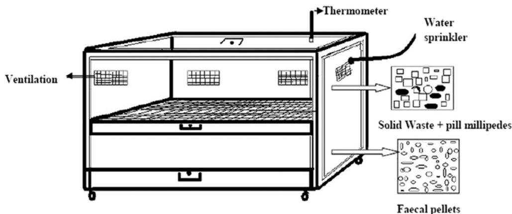
**Figure 2.** Improved bin model useful for compost production by pill millipedes.
