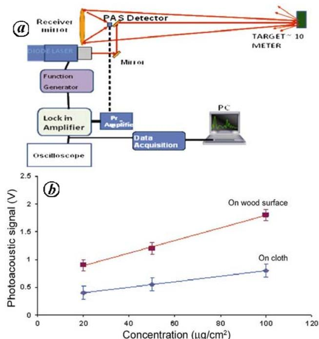
**Figure 3.** a, Standoff QE-LPAS set-up. b, Standoff normalized LPAS signal versus concentration of chlorophyll for target materials: wood and cloth.
