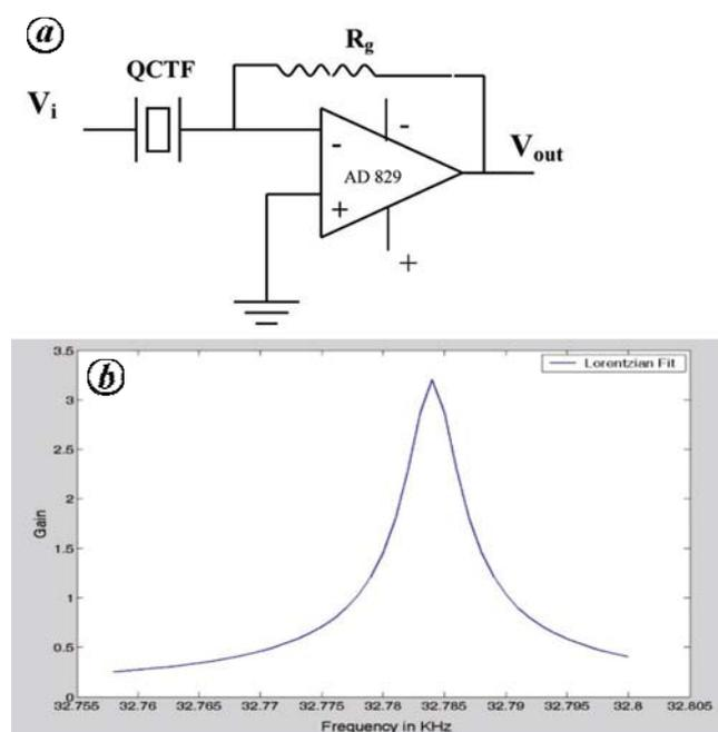
**Figure 1.** a, Trans-impedance amplifier circuit. b, Gain versus input frequency of QCTF.
