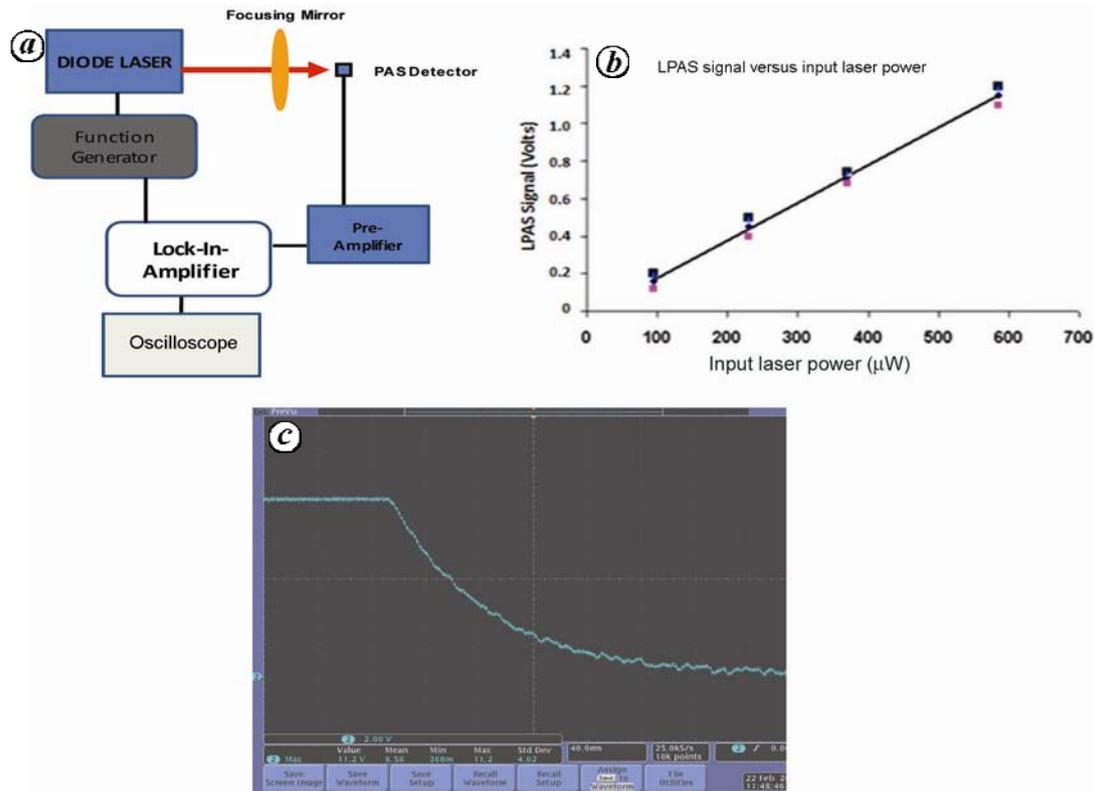
**Figure 2.** *a*, Optical set-up for QCTF detector. *b*, Optical characterization of QCTF detector. *c*, Detector voltage versus time (ms) (oscilloscope trace).
