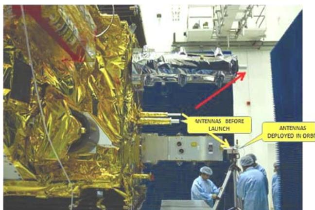
**Figure 4.** Deployment tests of ROSA antennas. The arrows indicate positions of spacecraft antennas after deployment; box shows body-mounted antennas before deployment.
