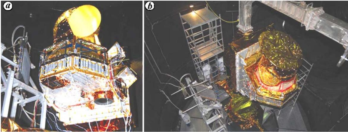
**Figure 2.** *a*, MADRAS undergoing thermo-vac tests in LSSC. *b*, MADRAS integration in LSSC before testing.
