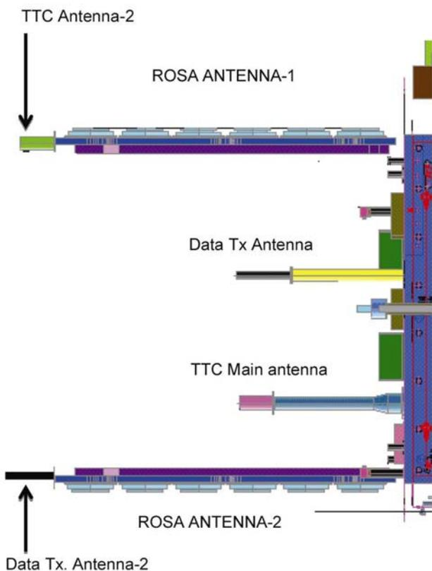
**Figure 3.** Data transmitter antenna 2 and TTC antenna 2 deployed in orbit.
