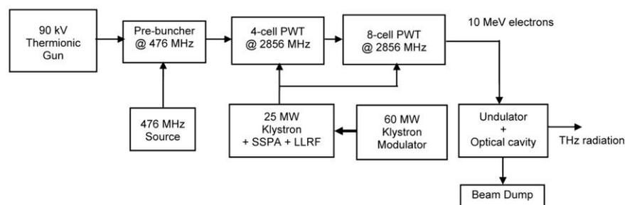
Figure 1. Schematic of the CUTE-FEL set-up.
