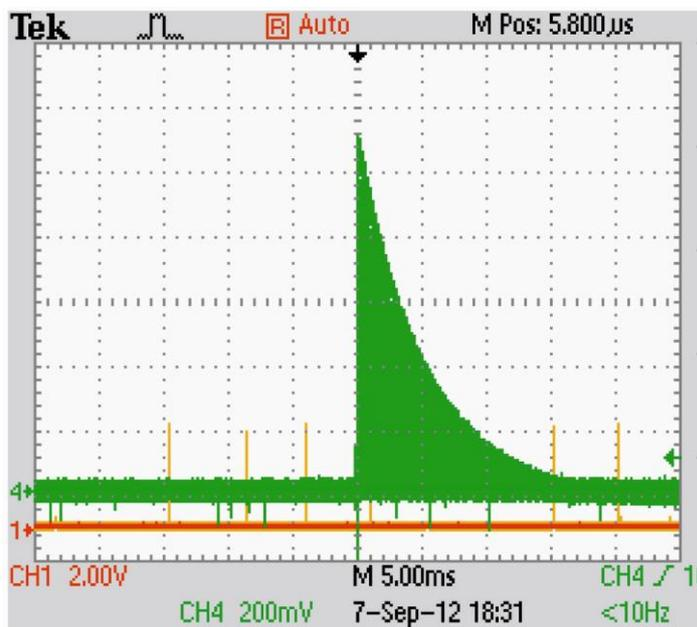
Figure 6. Bolometer trace of the measured out-coupled THz power.
