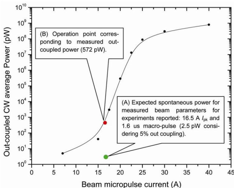
**Figure 4.** Expected variation of out-coupled THz power with beam current for a 7 MeV electron beam.
