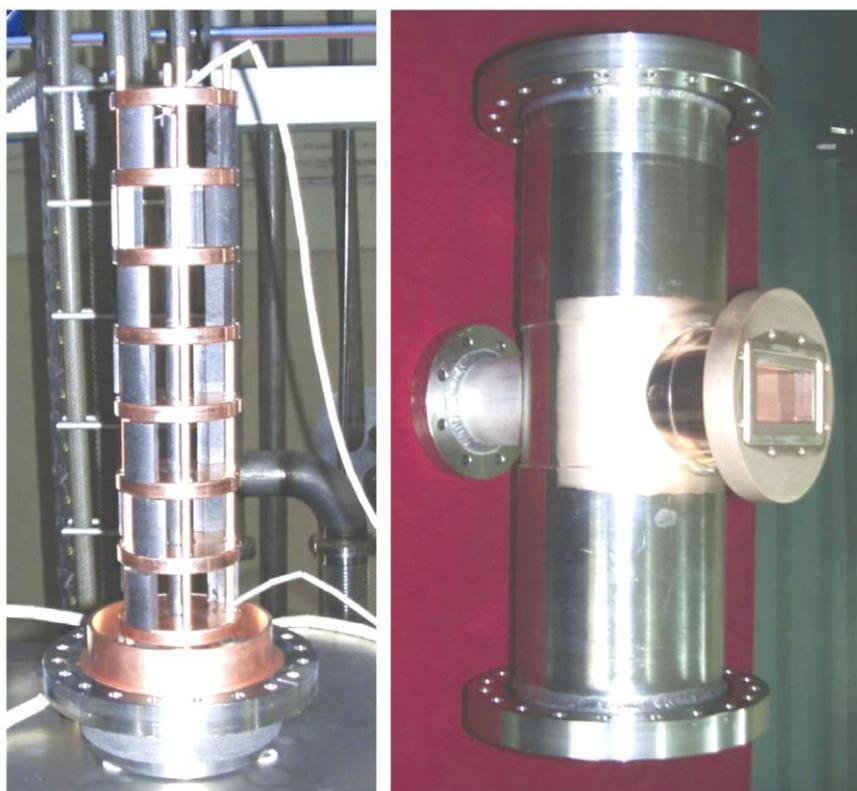
Figure 2. Disk array and tank envelope of 8-cell PWT linac just after brazing.
