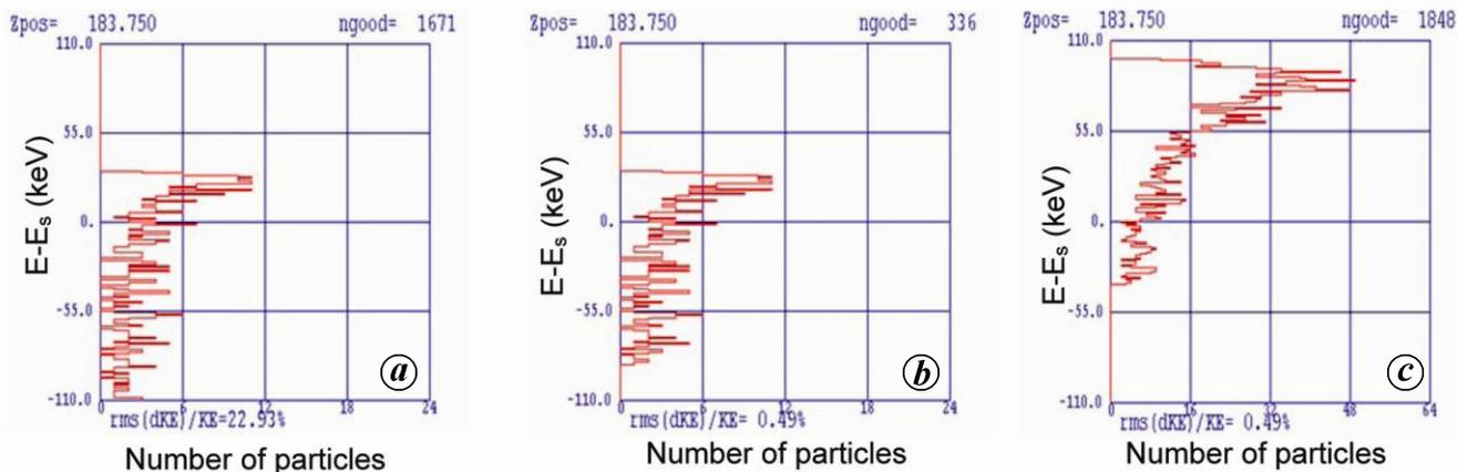
**Figure 3.** Electron beam energy spectrum at exit of eight cell PWT linac: (a) Total accelerated charge for stage-1 experiments with-out pre-buncher. (b) Fraction of accelerated charge within  $\delta E/E \leq 0.5\%$  for stage-1 experiments without pre-buncher and (c) Fraction of accelerated charge within  $\delta E/E \leq 0.5\%$  for stage-2 experiments.
