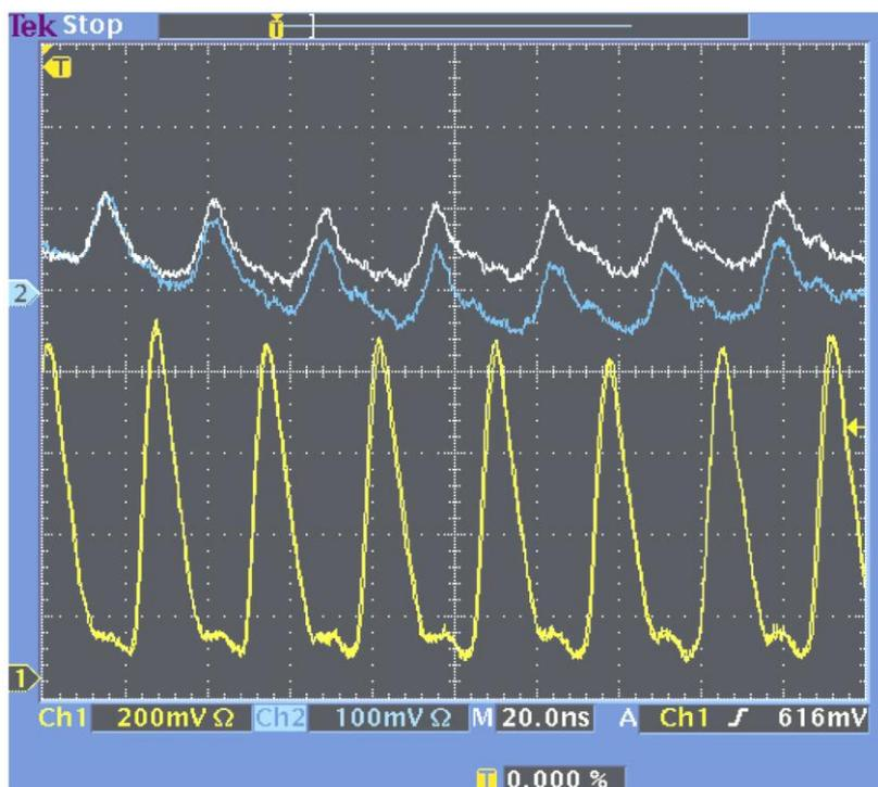
Figure 5. ICT traces of the electron beam: yellow, before and blue, after the linac.
