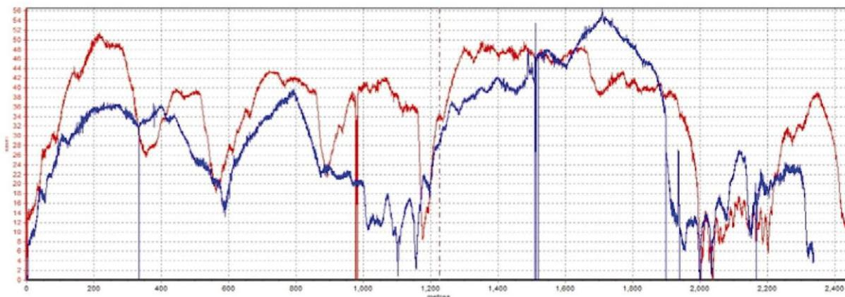
**Figure 2.** Speed profile before peak hour (red colour) and during peak hour (blue colour) on working days.
