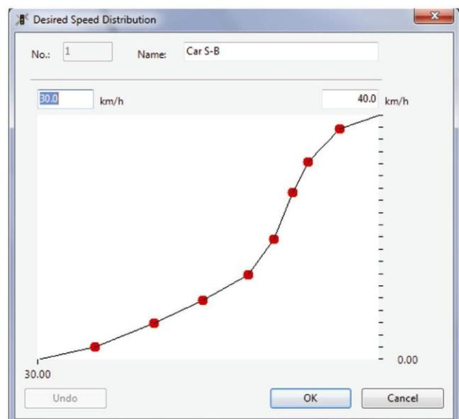
Figure 5. Typical desired speed distribution for car given in VISSIM.
