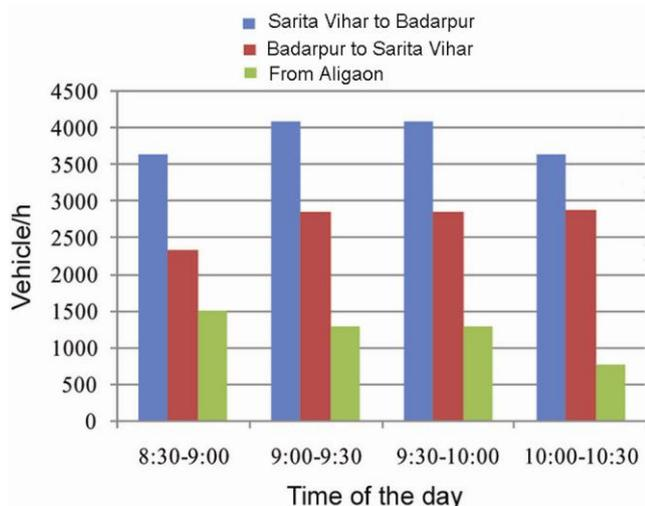
**Figure 7.** Vehicle flow provided as input in VISSIM.
