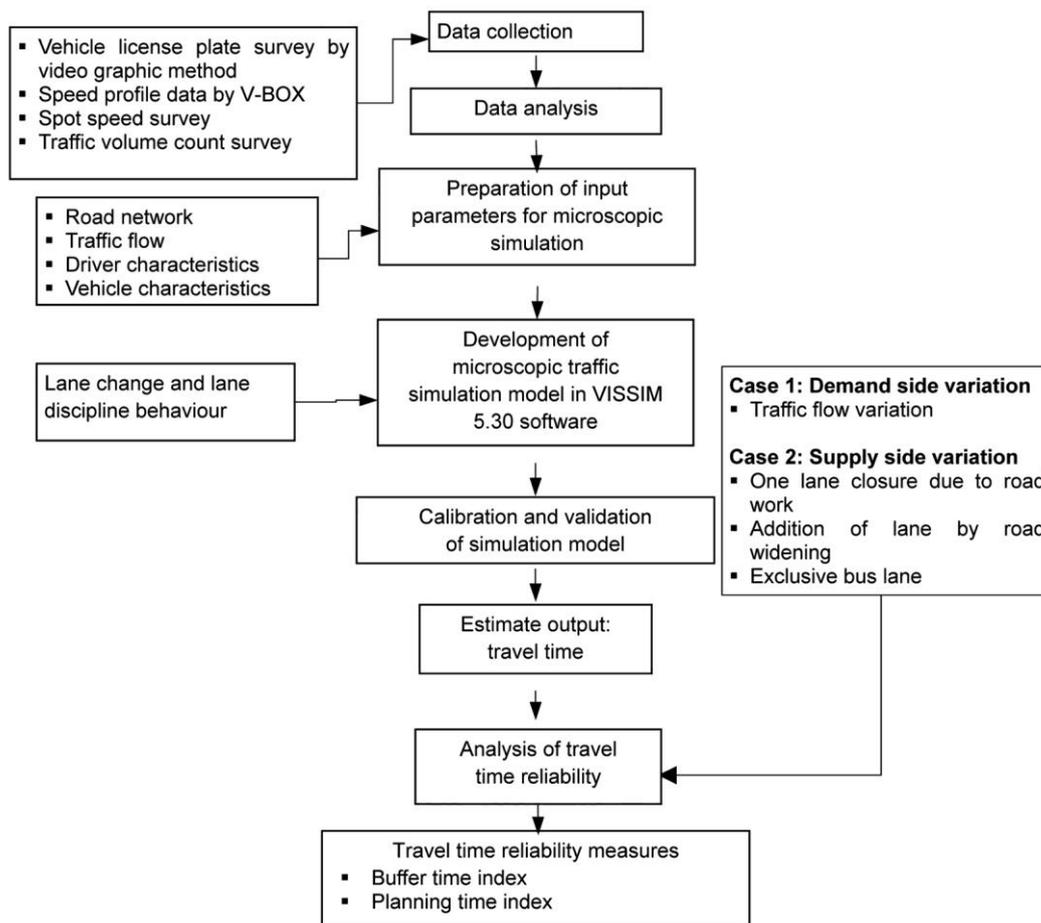
Figure 3. Adopted methodology for developing micro simulation model to analyse travel time reliability.
