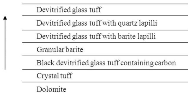
Figure 2. Geological succession of the Mangampeta barite deposit (after Kurien *et al.*<sup>3</sup>).
