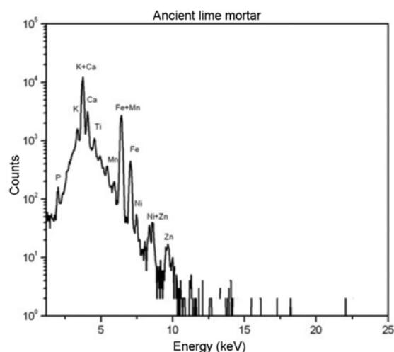
Figure 6. Particle-induced X-ray emission spectrum obtained by 3 MeV proton beam bombardment on sample showing trace elements.
