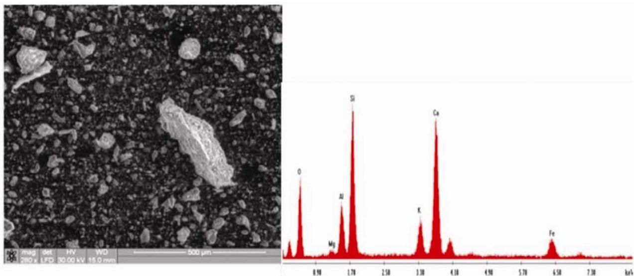
**Figure 2.** Scanning electron microscopy (SEM) coupled with energy dispersive X-ray spectra of ancient lime mortars highlighting binder aggregate matrix (280× magnification) with elemental composition of the surface layer.
