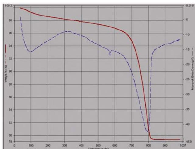
Figure 5. Thermogravimetric and differential thermal analysis curve of ancient lime mortar.
