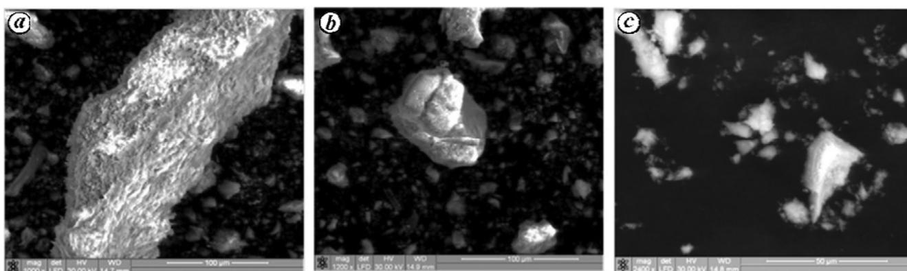
**Figure 3.** SEM observations of ancient lime mortar samples regarding the study of microstructural characteristics. *a*, Binder of sample scale bar length = 100 μm and magnification 1000×. *b*, Big grains of binder (calcite) of sample scale bar length = 100 μm and magnification 1200×. *c*, Binder (Ca) and silica (Si) particles on scale bar length = 50 μm and magnification 2400×.
