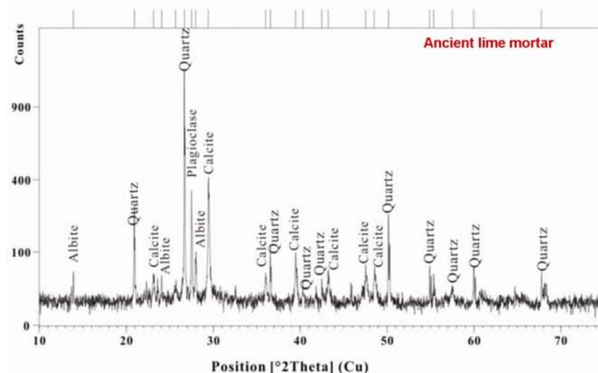
Figure 4. X-ray diffraction pattern of the historic lime mortar.
