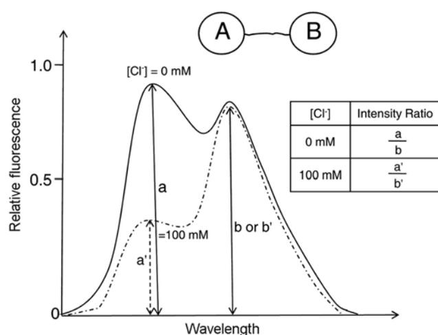
**Figure 2.** Fluorescence intensity ratio. The fluorescence emission spectrum of probe A is sensitive to chloride concentration in surrounding medium, while that of probe B is not. Intensity ratio from the covalently linked pair A–B can serve as an indicator of intracellular chloride ion concentration that is independent of the concentration of A–B.
