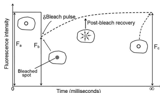
**Figure 5.** Fluorescence recovery after photobleaching. The typical variation in fluorescence intensity collected from a bleach spot with time during a spot photobleaching experiment is shown. A pictorial representation of the bleach zone at different times highlighting diffusion is also shown. See Figure 10 for comparison of bleach zone profile in TIR-FRAP and spot photobleaching.
