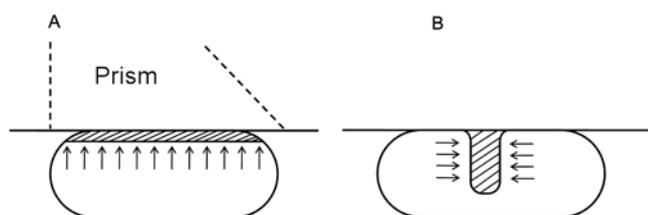
**Figure 10.** Bleach spot geometry. A, Shallow depth of TIR-FRAP bleach spot near the membrane owing to decaying evanescent field. The arrows highlight diffusion of unbleached fluorophores to the bleached zone. B, Deep cylindrical well of bleached fluorophores created by spot photobleaching. Fluorescence recovery at the bleached spot by two-dimensional diffusion of unbleached fluorophores is indicated by arrows.
