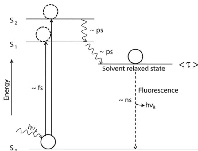
**Figure 3.** Fluorescence lifetime, i.e. the average time  $\langle \tau \rangle$  spent by a fluorophore in the excited state (typically 0.1–10 ns).
