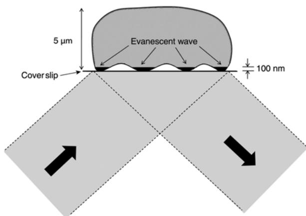
**Figure 8.** TIR excitation at membrane adjacent cytoplasm. TIR fluorescence image can reveal the distinct regions of focal contacts in the cell shown here. Selective excitation of fluorophores near the membrane interface is made possible by the exponential decay of the evanescent field in  $z$ -axis.
