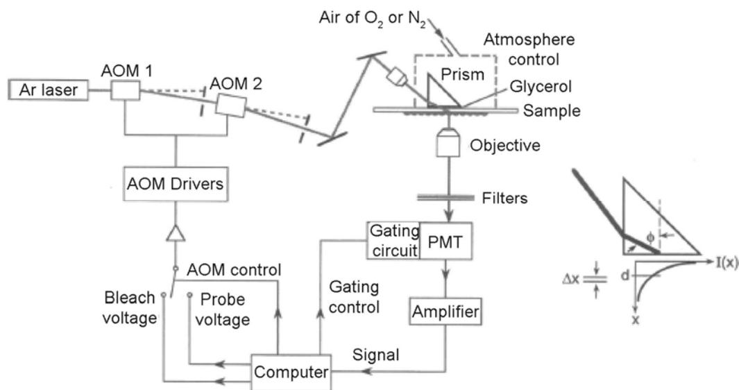
**Figure 9.** (Left) Schematic of TIR-FRAP instrumentation. The beam from an Ar ion laser was modulated by serial acousto-optic modulators and directed onto the sample through a 25X objective lens and right triangular fused silica prism. The signal was filtered and detected by a gated photomultiplier. (Right) Expanded view of prism showing beam incident angle,  $\phi$  and evanescent field depth,  $d$ . Reprinted with permission from ref. 94.
