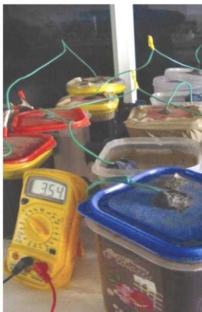
Figure?????? Stacked microbial fuel cells showing 3.54 V.
