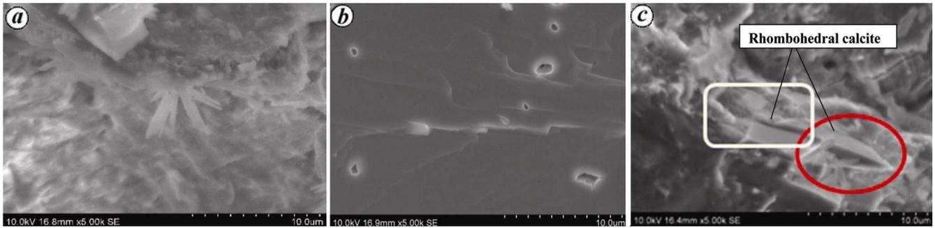
**Figure 2.** SEM images of bacteria incorporated mortar samples. *a*, MTCC 1761 incorporated mortar with cell concentration of  $10^5$  cells/ml. *b*, Bacterial impressions on the mortar surface of MTCC type. *c*, Rhombohedral calcite precipitation for the samples of CS-I incorporated mortar with cell concentration of  $10^6$  cells/ml.
