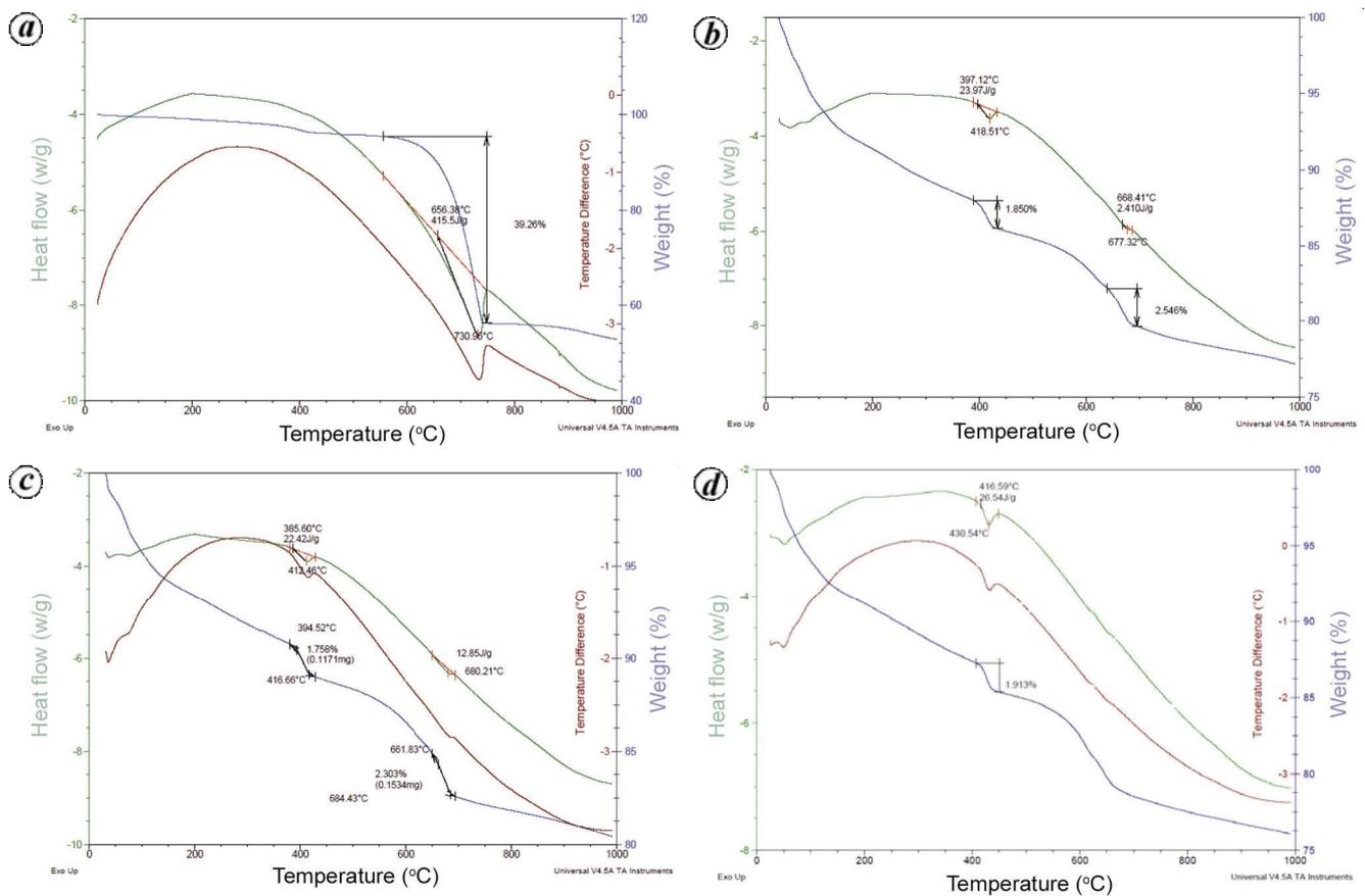
**Figure 3.** TGA graphs for (a) commercial calcite as reference, (b) MTCC 1761 sample, (c) CS-I sample and (d) control sample.
