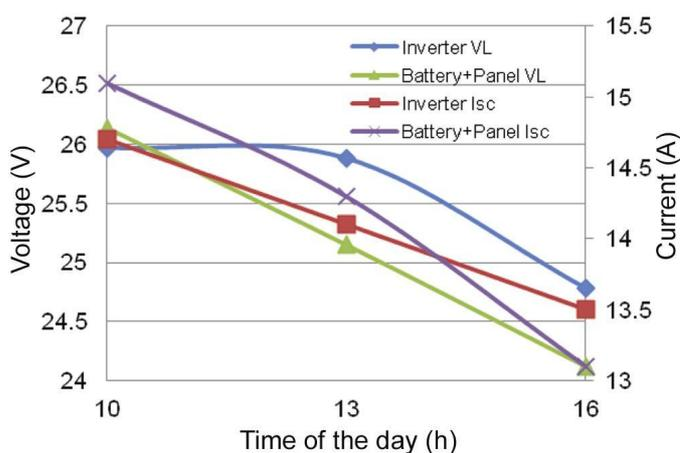
**Figure 3.** Variation of voltage and current at different times of the day.
