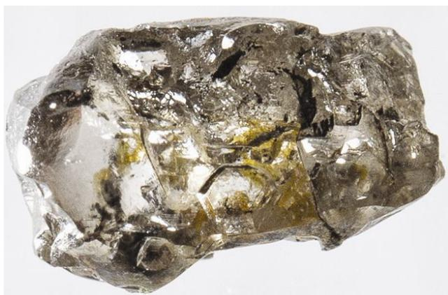
**Figure 1.** Enlarged image of impure diamond from Juína, Brazil (courtesy: Graham Pearson, University of Alberta). The diamond is 5 mm in long axis. A microscopic inclusion of ringwoodite, which is a high-pressure polymorph of mineral olivine [(Mg,Fe)<sub>2</sub>SiO<sub>4</sub>] was documented using Raman spectroscopy by Pearson *et al.*<sup>1</sup>.
