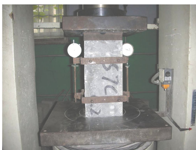
Figure 2. Testing apparatus of compressive modulus of elasticity.
