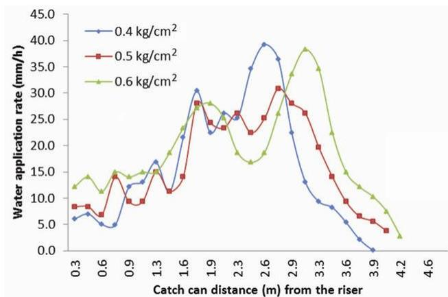
**Figure 3.** Water application rate of nozzle at different operating pressures.
