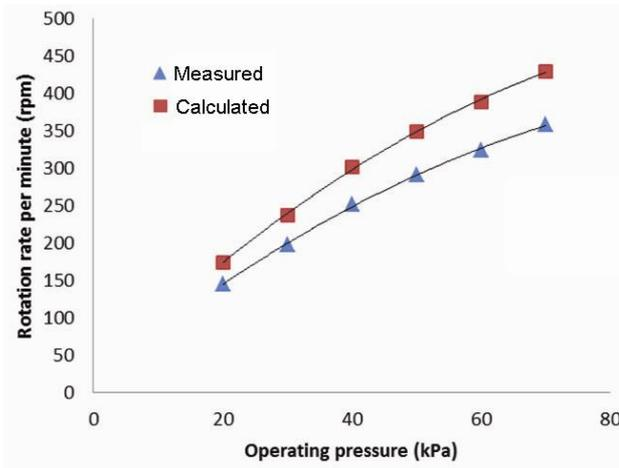
Figure 4. Rotational rate of nozzle at different operating pressures.
