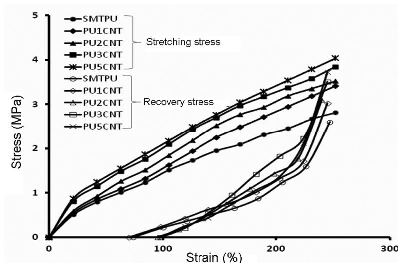
**Figure 2.** Stretching stresses as well as recovery stresses for 0, 1, 2, 3 and 5 phr MWCNT reinforced SMTPU.
