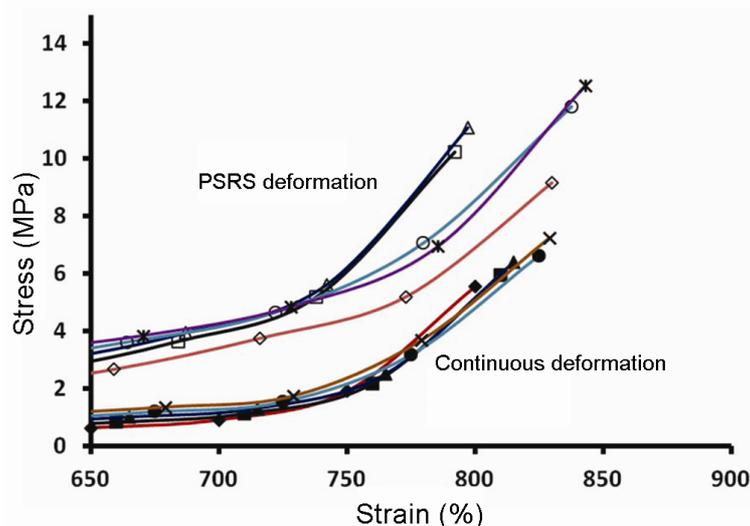
**Figure 3.** The recovery stresses at different strains for various deformed test samples using both conventional continuous stretching and PSRS scheme.
