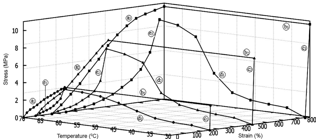
**Figure 1.** The steps involved in modified shape memory creation procedure, progressive stretch–relax–stretch (PSRS) scheme and shape memory effect determination illustrated by three-dimensional representative curves obtained experimentally for SMTPU.
