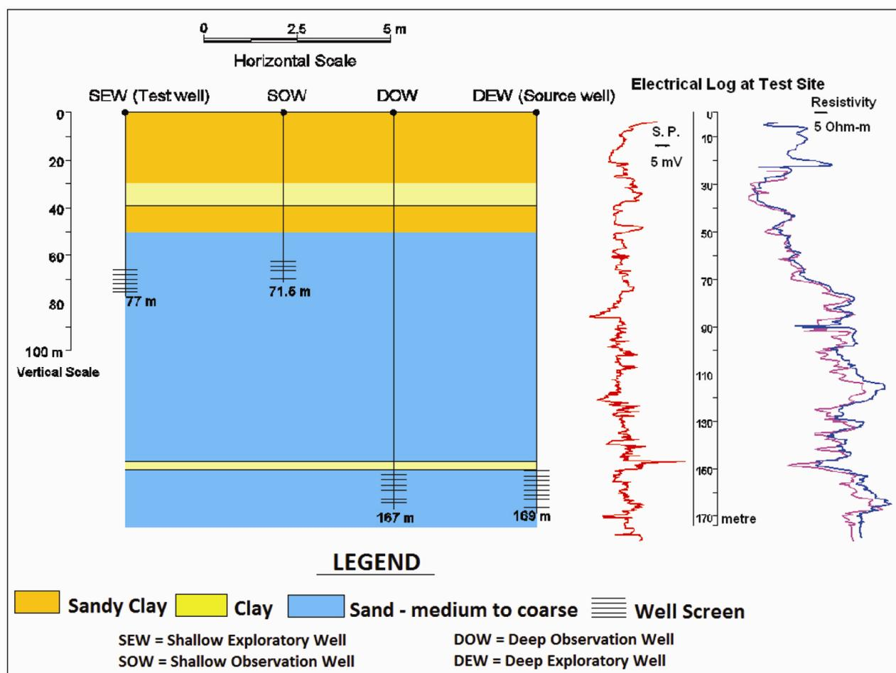
Figure 1. Schematic diagram showing the experimental set-up and electrical geophysical log at the test site.
