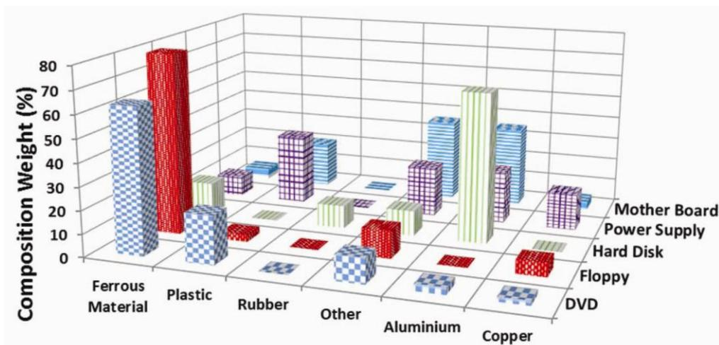
Figure 3. Per unit weight percentage of the materials from separated parts of CPU in PC.
